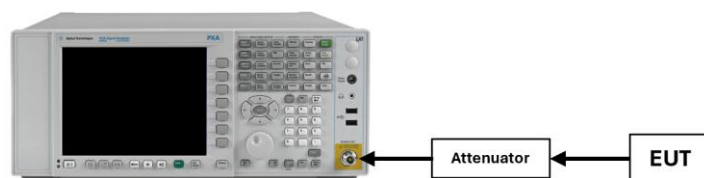
Figure 7-1. Test Instrument & Measurement Setup
