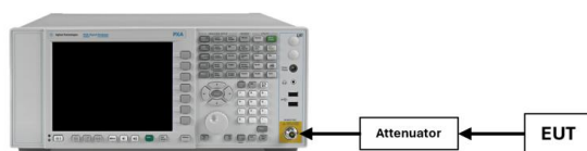
Figure 7-4. Test Instrument & Measurement Setup
