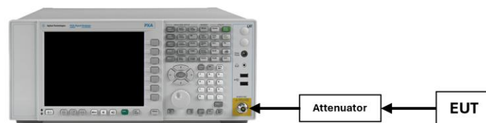
Figure 7-5. Test Instrument & Measurement Setup
