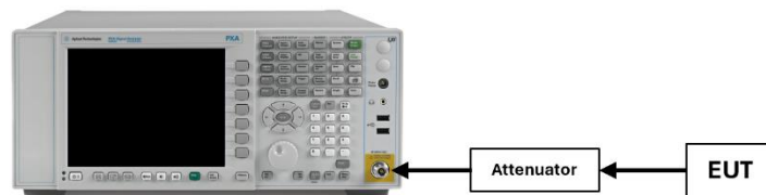
Figure 7-3. Test Instrument & Measurement Setup
