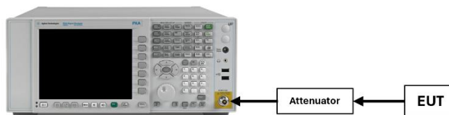
Figure 7-4. Test Instrument & Measurement Setup
