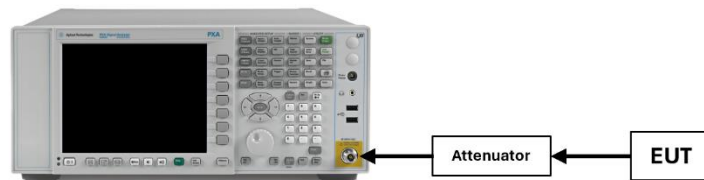
Figure 7-5. Test Instrument & Measurement Setup
