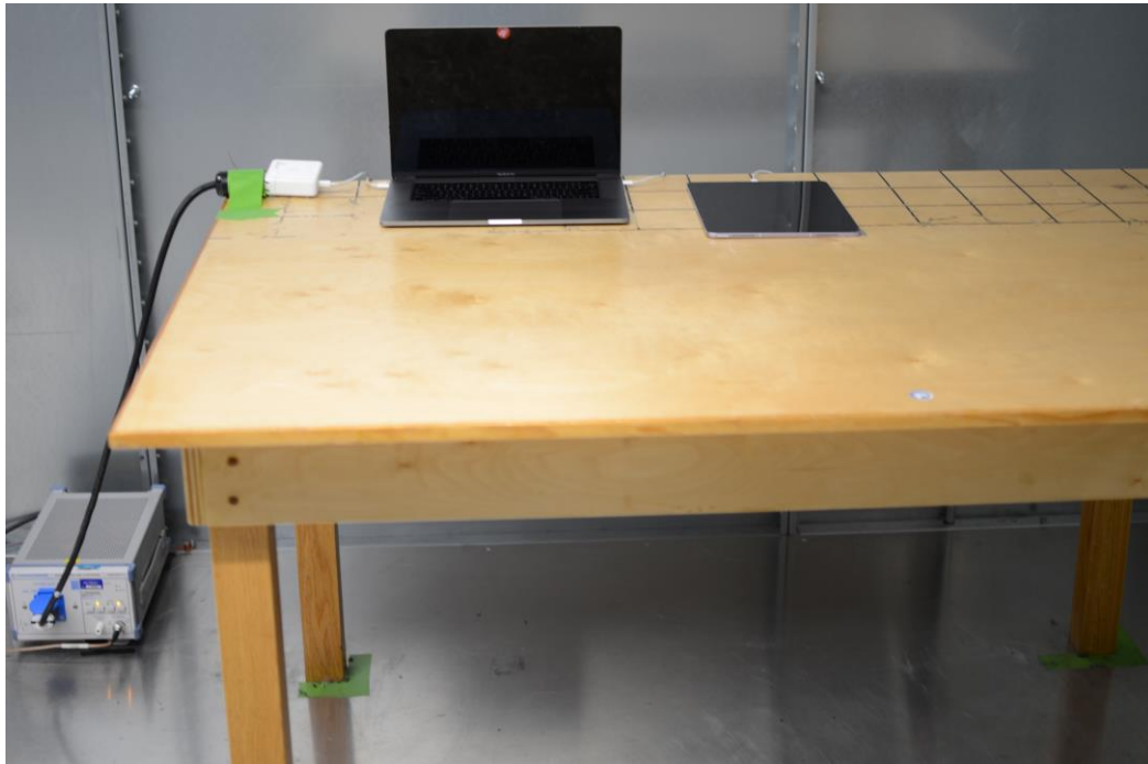
Figure 3: AC Line Conducted Emissions (Front View)
