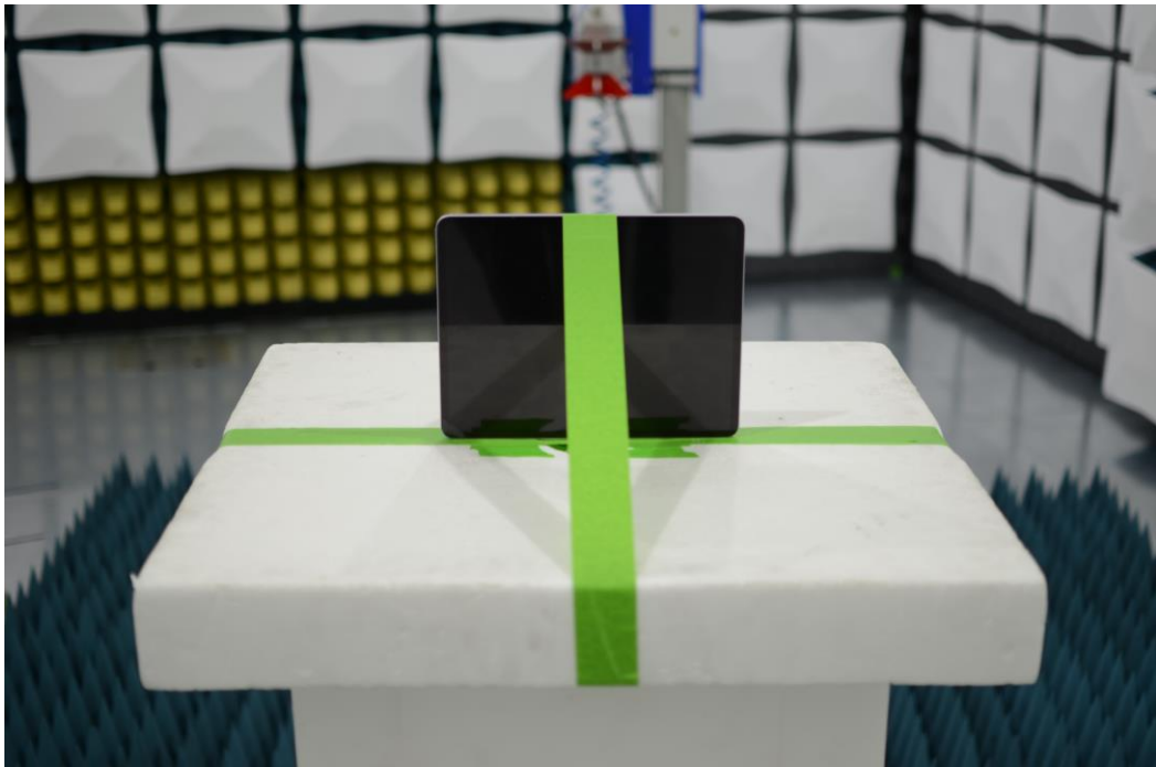
Figure 8: 1-18GHz Test Setup (Rear View)
