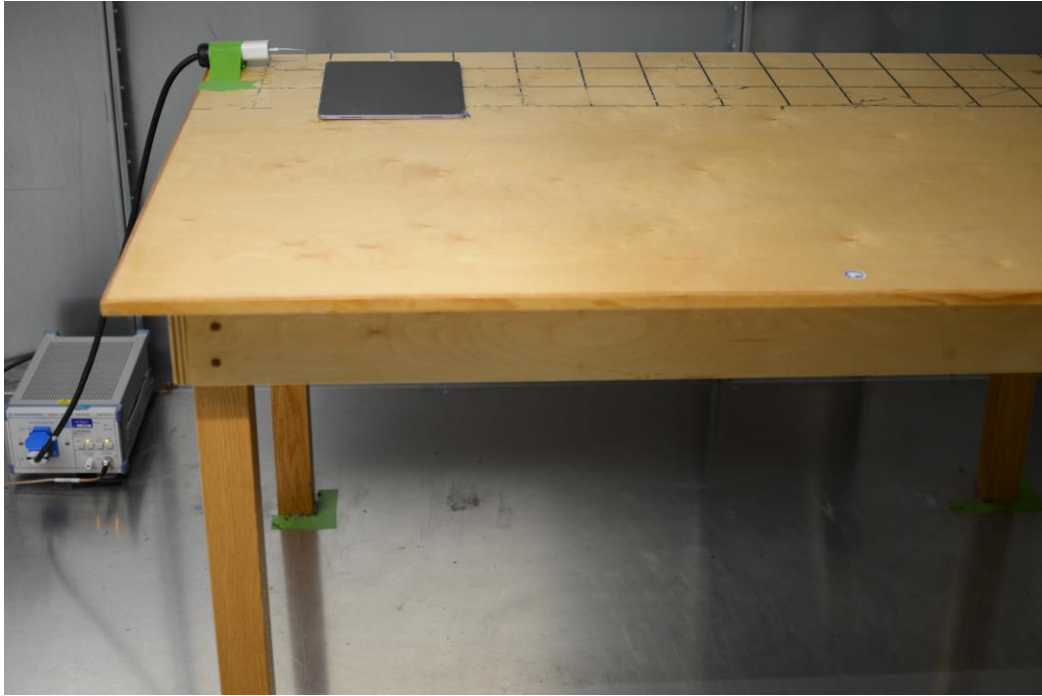
Figure 1: AC Line Conducted Emissions (Front View)
