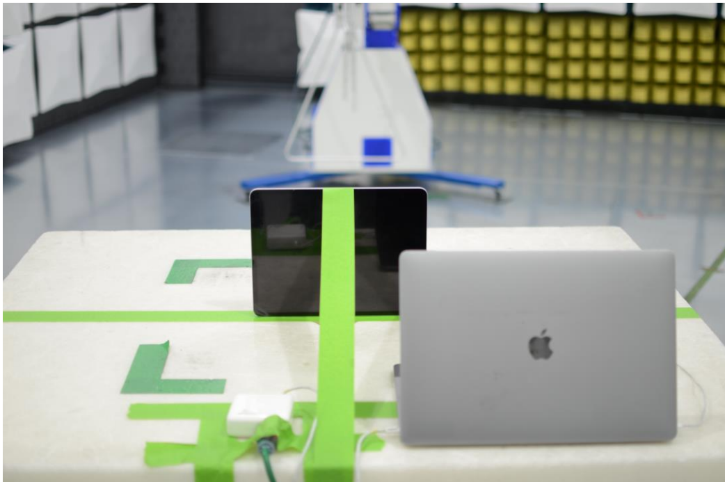
Figure 20: 30MHz-1GHz Test Setup (Rear View)
