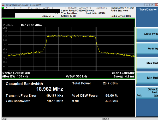
Plot 7-8. 6dB BW & 99% OBW Antenna 5T (20MHz BW 11ax– RU242 – Ch.157)
