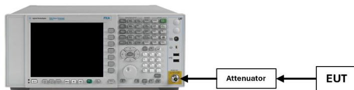
Figure 7-1. Test Instrument & Measurement Setup
