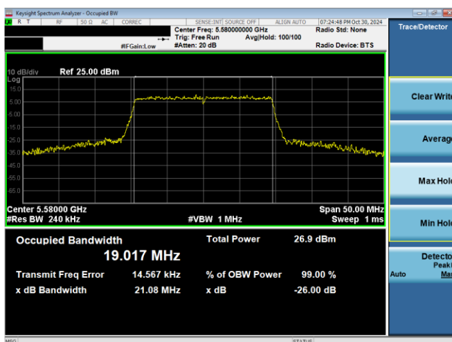
Plot 7-2. 26dB BW & 99% OBW Antenna 5T (20MHz BW 11ax – RU242 – Ch.116)
