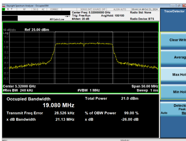
Plot 7-6. 26dB BW & 99% OBW Antenna 1b (20MHz BW 11ax – RU242 – Ch.64)
