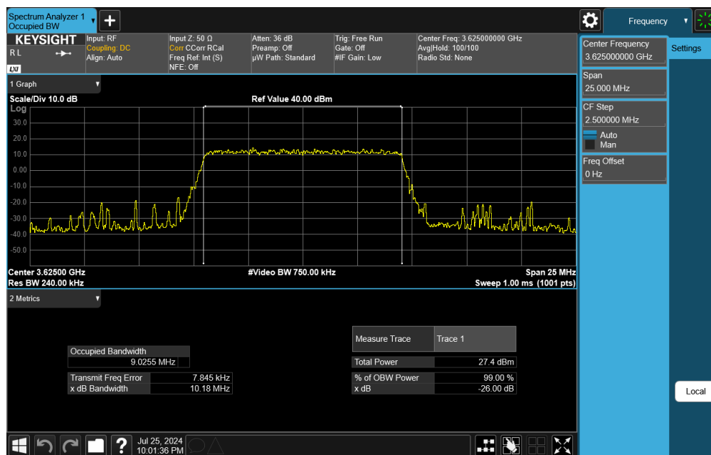
Plot 7-8. Occupied Bandwidth Plot (LTE Band 48 - 10MHz 256-QAM - Full RB Configuration)
