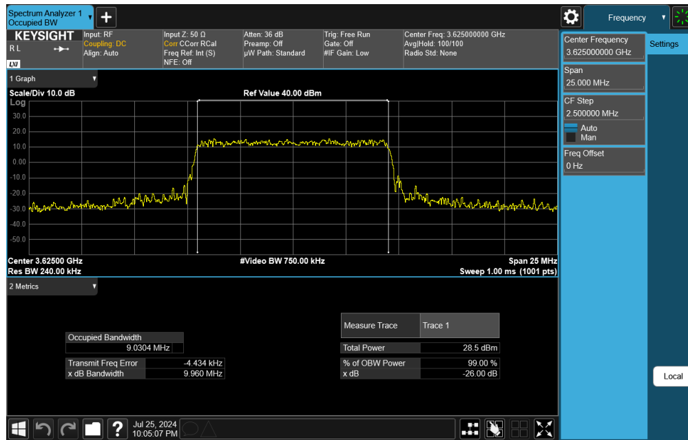
Plot 7-7. Occupied Bandwidth Plot (LTE Band 48 - 10MHz 64-QAM - Full RB Configuration)
