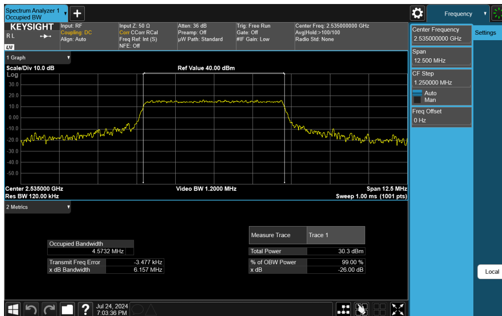
Plot 7-12. Occupied Bandwidth Plot (LTE Band 7 - 5MHz 256-QAM - Full RB)
