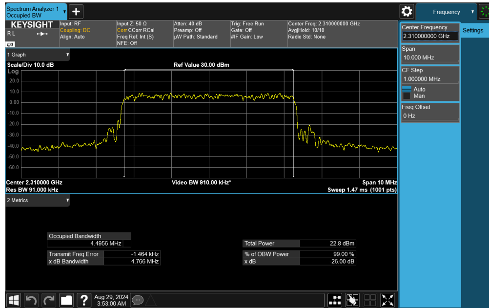
Plot 7-43. Occupied Bandwidth Plot (NR Band n30 - 5MHz CP-OFDM 16-QAM - Full RB)
