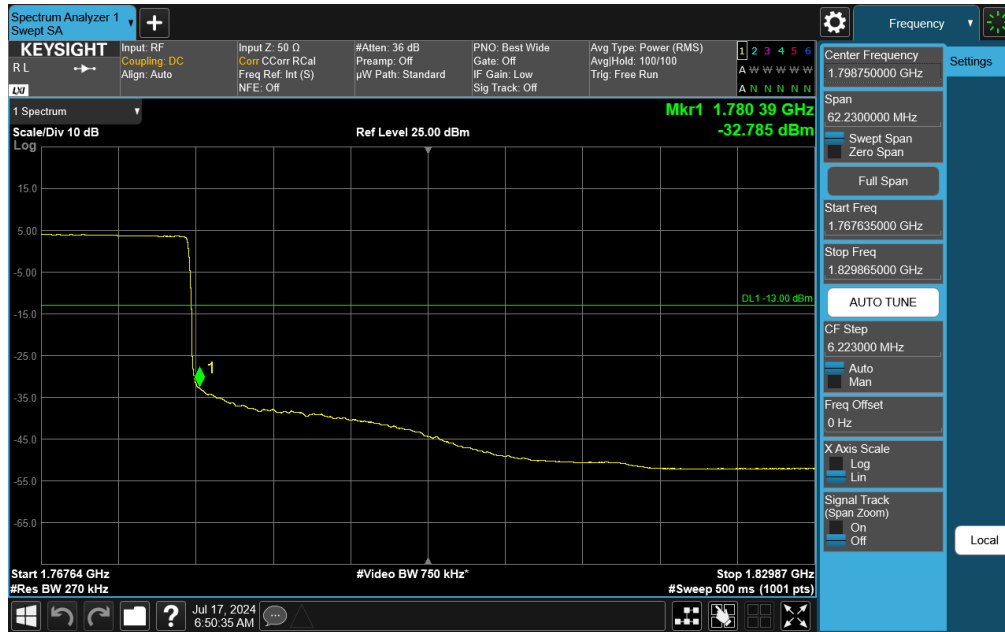
Plot 7-330. Upper Band Edge Plot (NR Band n66 – 25.0MHz CP-OFDM QPSK - Full RB)
