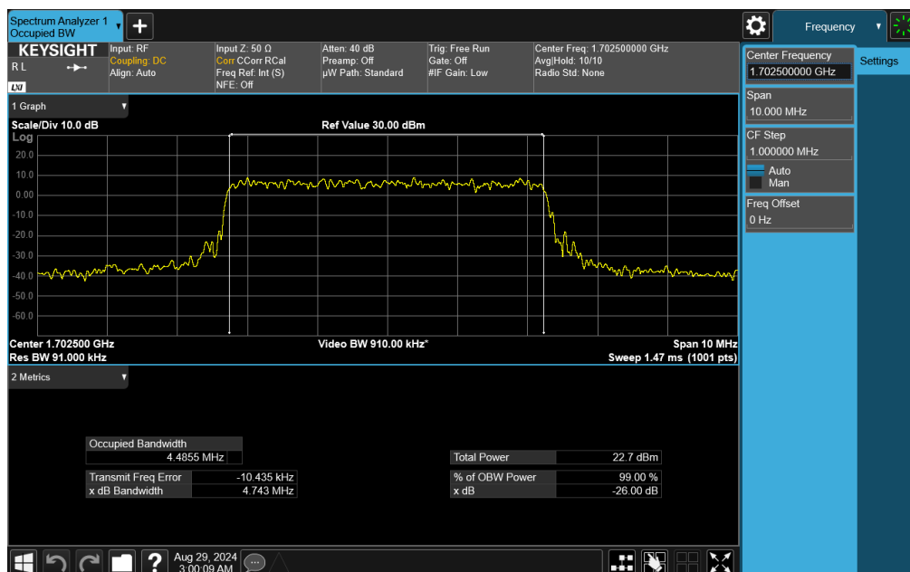
Plot 7-107. Occupied Bandwidth Plot (NR Band n70 - 5MHz CP-OFDM 16-QAM - Full RB)
