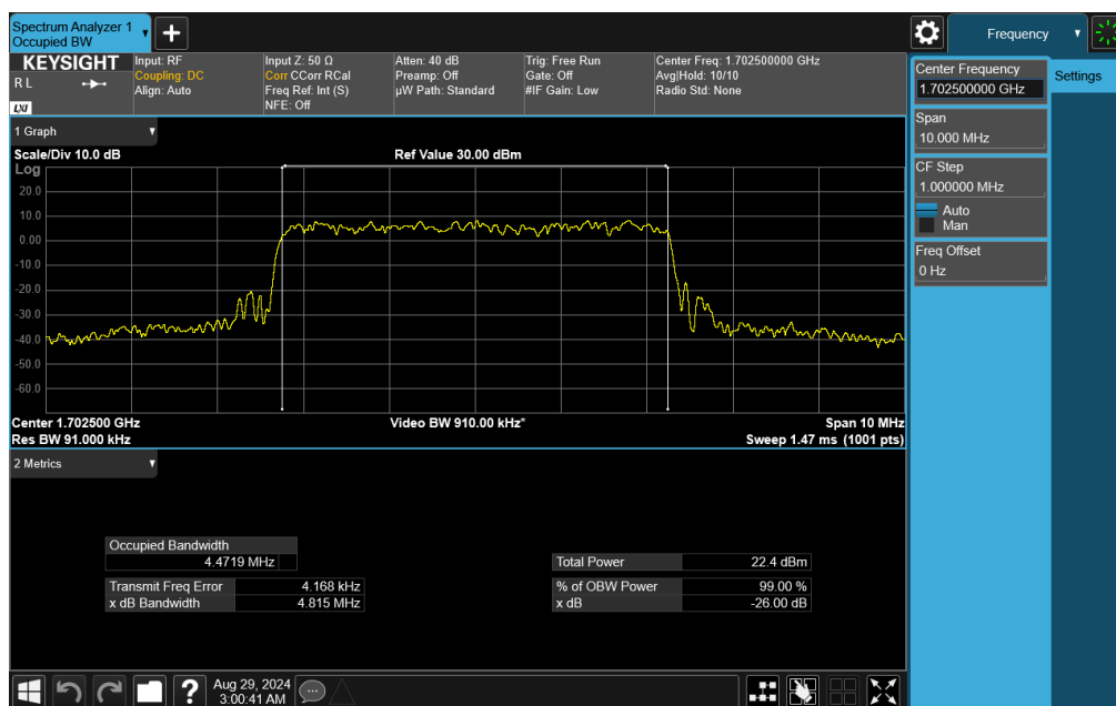
Plot 7-108. Occupied Bandwidth Plot (NR Band n70 - 5MHz CP-OFDM 64-QAM - Full RB)
