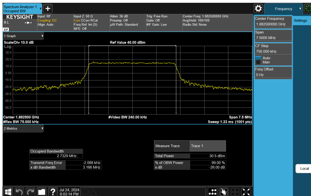
Plot 7-8. Occupied Bandwidth Plot (LTE Band 25/2 - 3MHz 256-QAM - Full RB Configuration)
