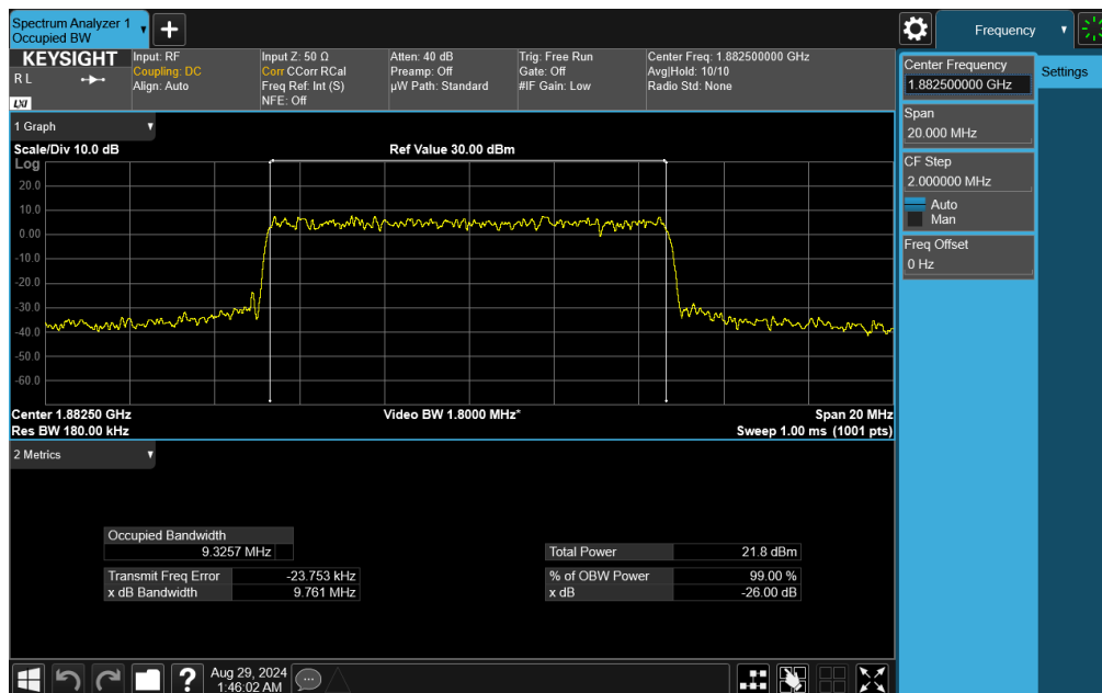
Plot 7-33. Occupied Bandwidth Plot (NR Band n25/n2 - 10MHz CP-OFDM 64QAM - Full RB)
