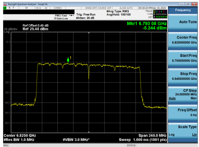
Plot 7-272. PSD Plot Antenna WF2a (160MHz 802.11ax RU26 (UNII Band 7) - Ch. 175)
