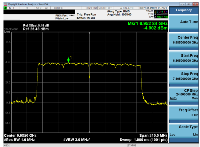
Plot 7-224. PSD Plot Antenna WF7a (160MHz 802.11ax RU996x2 (UNII Band 8) - Ch. 207)
