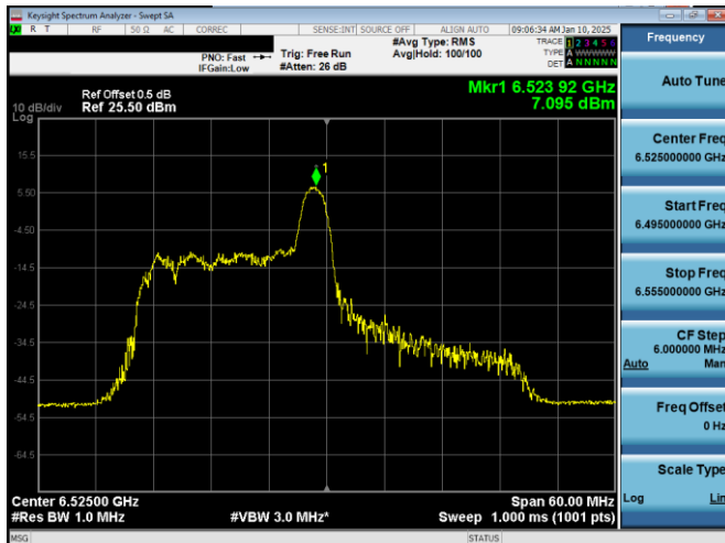
Plot 7-234. PSD Plot Antenna WF2a (40MHz 802.11ax RU26 (UNII Band 6) – Ch. 115)
