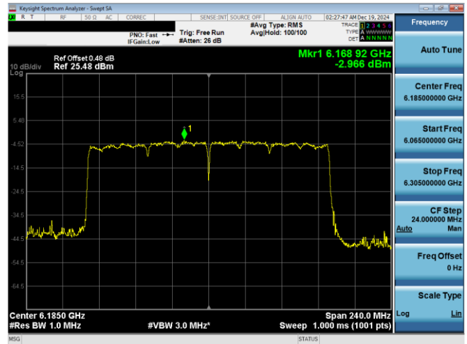
Plot 7-200. PSD Plot Antenna WF7a (160MHz 802.11ax RU996x2 (UNII Band 5) – Ch. 47)
