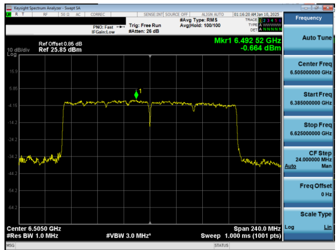
Plot 7-184. PSD Plot Antenna WF7a (160MHz 802.11ax RU996x2 (UNII Band 6) - Ch. 111)
