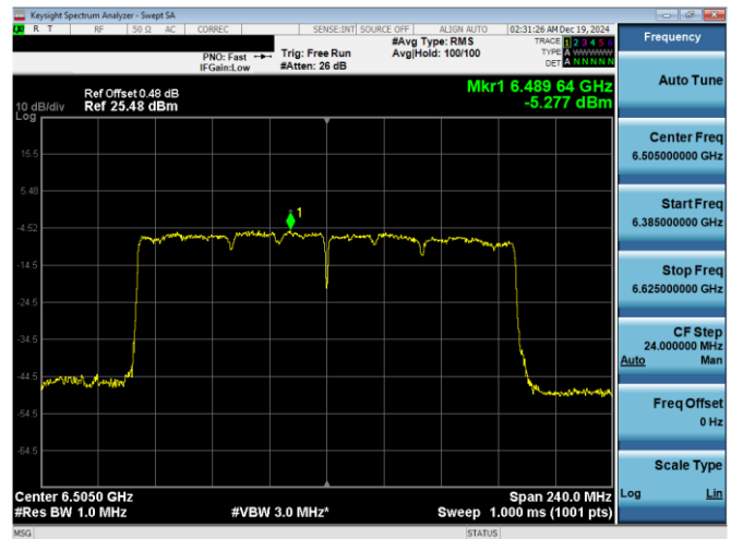
Plot 7-208. PSD Plot Antenna WF7a (160MHz 802.11ax RU996x2 (UNII Band 6) - Ch. 111)
