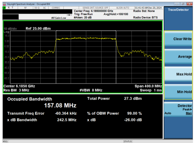
Plot 7-144. 26dB & 99% Bandwidth Plot Antenna WF7b (160MHz 802.11ax RU996x2 (UNII Band 5) – Ch. 47)
