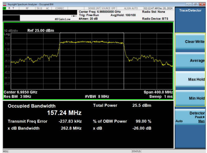
Plot 7-168. 26dB & 99% Bandwidth Plot Antenna WF7b (160MHz 802.11ax RU996x2 (UNII Band 8) – Ch. 207)
