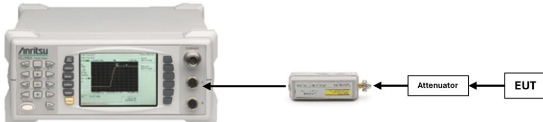
Figure 7-2. Test Instrument & Measurement Setup
