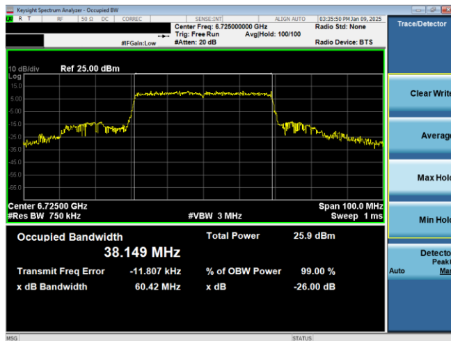
Plot 7-22. 26dB & 99% Bandwidth Plot Antenna WF7a (40MHz 802.11ax RU484 (UNII Band 7) – Ch. 155)
