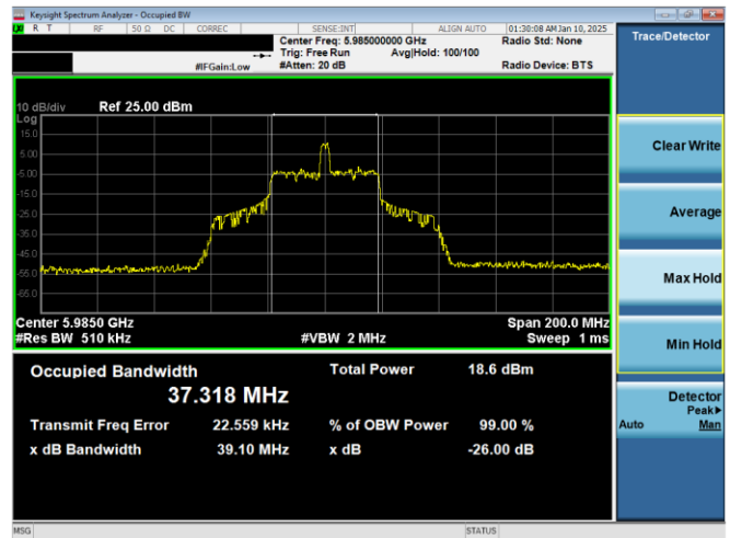
Plot 7-59. 26dB & 99% Bandwidth Plot Antenna WF2a (80MHz 802.11ax RU26 (UNII Band 5) – Ch. 7)
