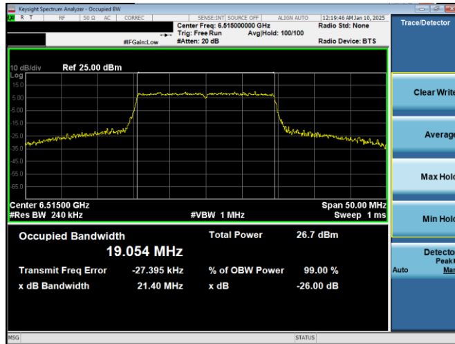
Plot 7-13. 26dB & 99% Bandwidth Plot Antenna WF7a (20MHz 802.11ax RU242 (UNII Band 6) – Ch. 113)
