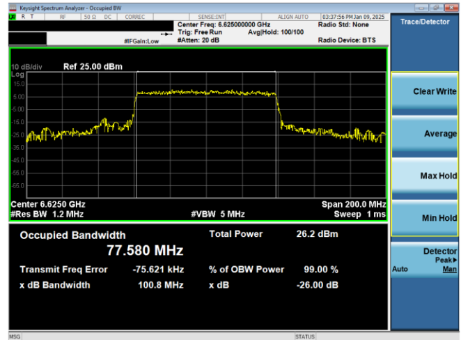
Plot 7-23. 26dB & 99% Bandwidth Plot Antenna WF7a (80MHz 802.11ax RU996 (UNII Band 7) – Ch. 135)
