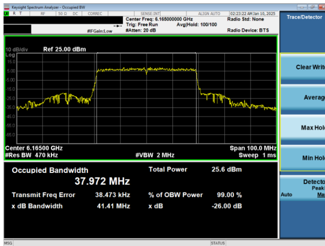
Plot 7-62. 26dB & 99% Bandwidth Plot Antenna WF2a (40MHz 802.11ax RU484 (UNII Band 5) – Ch. 43)
