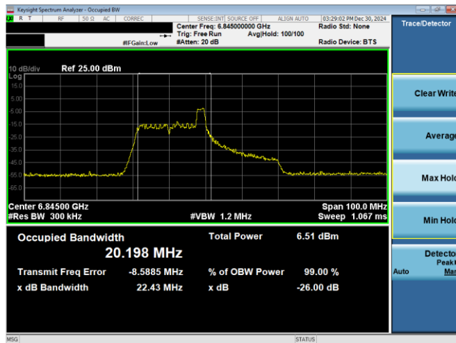
Plot 7-42. 26dB & 99% Bandwidth Plot Antenna WF7a (40MHz 802.11ax RU26 (UNII Band 7) – Ch. 179)
