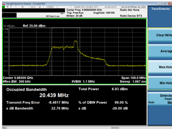
Plot 7-26. 26dB & 99% Bandwidth Plot Antenna WF7a (40MHz 802.11ax RU26 (UNII Band 5) – Ch. 3)
