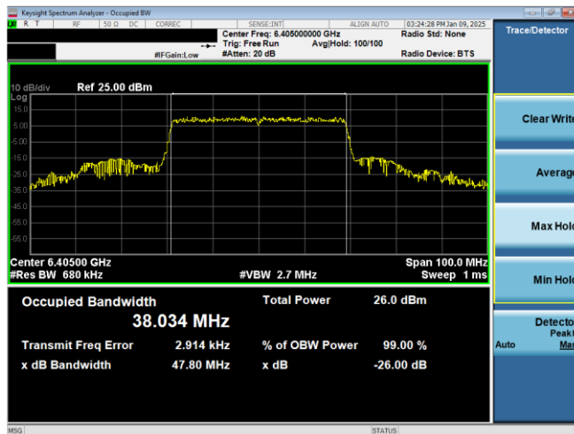
Plot 7-6. 26dB & 99% Bandwidth Plot Antenna WF7a (40MHz 802.11ax RU484 (UNII Band 5) – Ch. 91)
