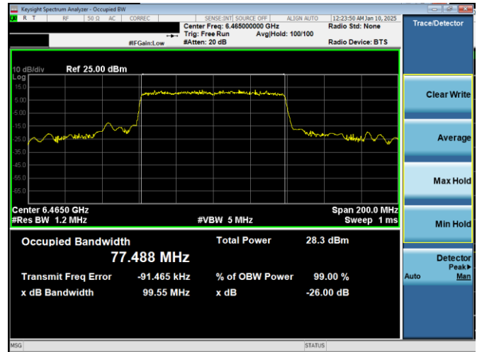
Plot 7-15. 26dB & 99% Bandwidth Plot Antenna WF7a (80MHz 802.11ax RU996 (UNII Band 6) – Ch. 103)
