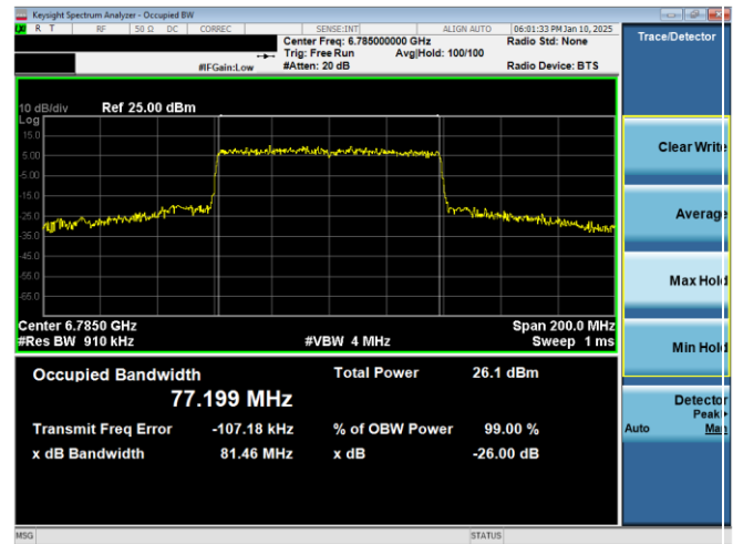
Plot 7-67. 26dB & 99% Bandwidth Plot Antenna WF7b (80MHz 802.11ax (UNII Band 7) – Ch. 167)
