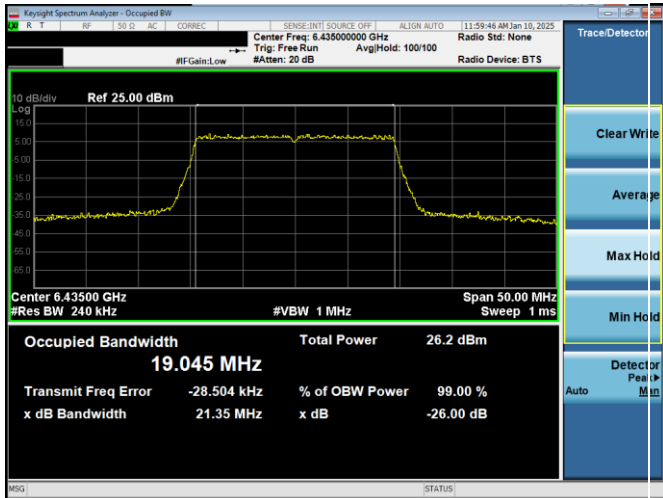
Plot 7-61. 26dB & 115% Bandwidth Plot Antenna WF7b (20MHz 802.11ax (UNII Band 6) – Ch. 97)
