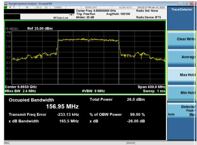
Plot 7-68. 26dB & 99% Bandwidth Plot Antenna WF7b (160MHz 802.11ax (UNII Band 7) – Ch. 143)
