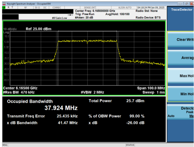
Plot 7-2. 26dB & 99% Bandwidth Plot Antenna WF7a (40MHz 802.11ax (UNII Band 5) – Ch. 43)
