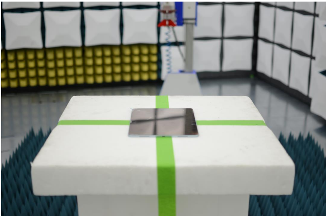
Figure 6: 1-18GHz Test Setup (Rear View)
