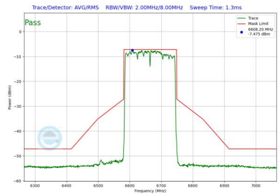
Plot 7-172. In-Band Emission Plot Antenna 3c (160MHz 802.11ax RU996x2 (UNII Band 7) – Ch. 143)
