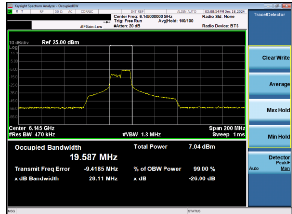
Plot 7-19. 26dB & 99% Bandwidth Plot Antenna 3a (80MHz 802.11ax RU106 (UNII Band 5) – Ch. 39)
