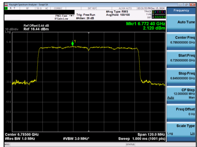
Plot 7-493. PSD Plot SDM Diversity Antenna 3c (80MHz 802.11ax RU996 (UNII Band 7) – Ch. 167)
