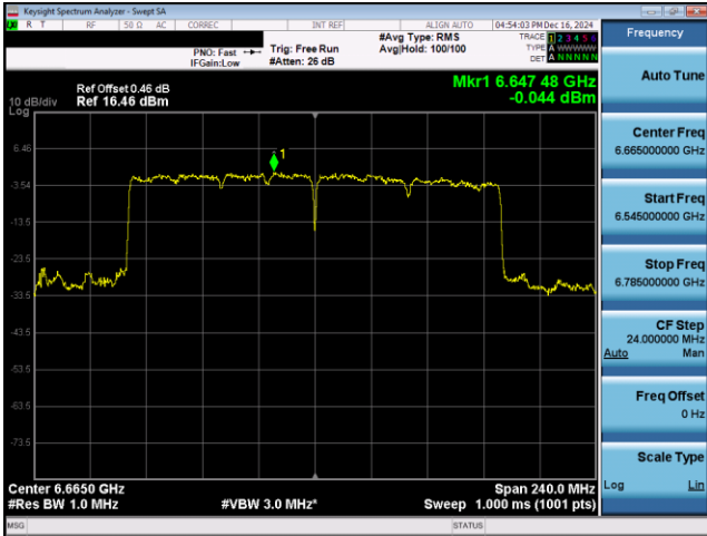
Plot 7-496. PSD Plot SDM Diversity Antenna 1b (160MHz 802.11ax RU996x2 (UNII Band 7) – Ch. 143)
