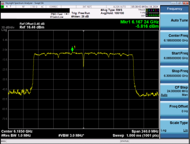
Plot 7-512. PSD Plot SDM Diversity Antenna 1b (160MHz 802.11ax RU996x2 (UNII Band 5) – Ch. 47)
