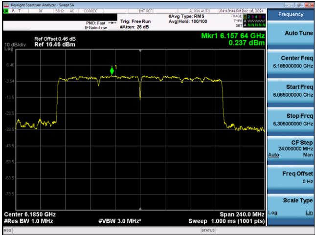
Plot 7-464. PSD Plot CDD Diversity Antenna 1b (160MHz 802.11ax RU996x2 (UNII Band 5) – Ch. 47)
