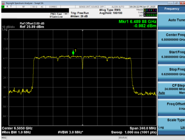
Plot 7-367. PSD Plot CDD Antenna 3c (160MHz 802.11ax RU996x2 (UNII Band 6) – Ch. 111)
