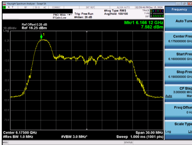
Plot 7-337. PSD Plot CDD Primary Antenna 3c (20MHz 802.11ax RU26 (UNII Band 5) – Ch. 45)
