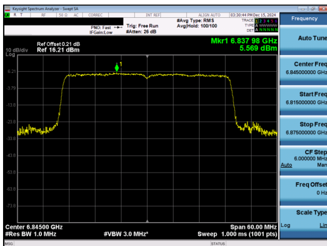
Plot 7-379. PSD Plot CDD Primary Antenna 3c (40MHz 802.11ax RU484 (UNII Band 7) – Ch. 179)
