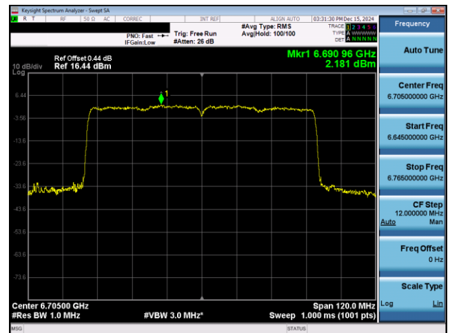
Plot 7-381. PSD Plot CDD Primary Antenna 3c (80MHz 802.11ax RU996 (UNII Band 7) – Ch. 151)
