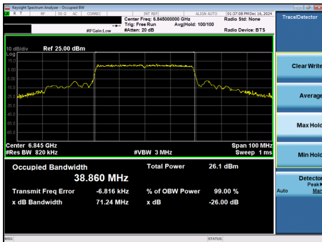
Plot 7-134. 26dB & 99% Bandwidth Plot Antenna 1b (40MHz 802.11ax RU484 (UNII Band 7) – Ch. 179)
