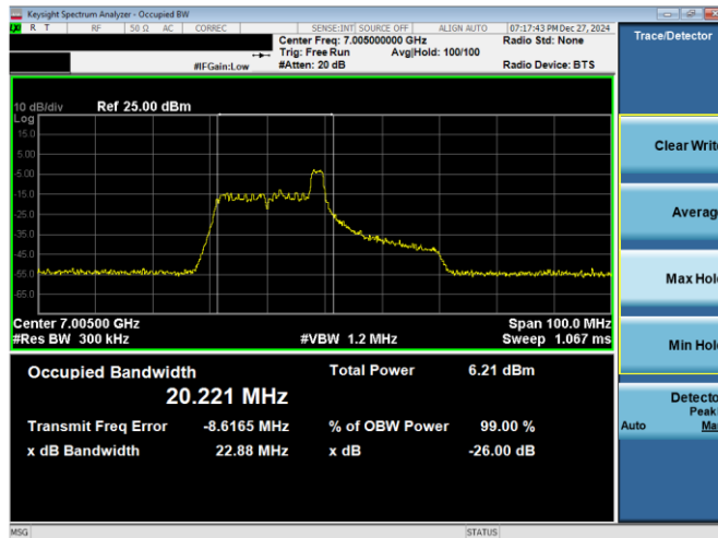
Plot 7-162. 26dB & 99% Bandwidth Plot Antenna 1b (40MHz 802.11ax RU26 (UNII Band 8) – Ch. 211)
