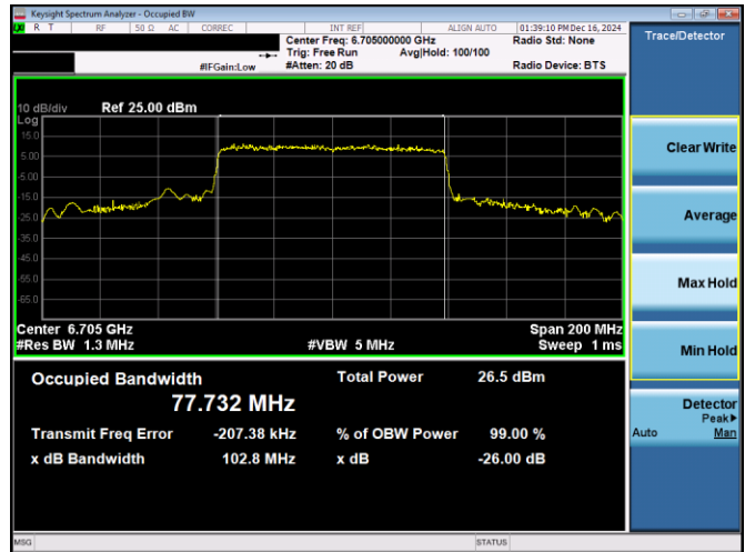
Plot 7-135. 26dB & 99% Bandwidth Plot Antenna 1b (80MHz 802.11ax RU996 (UNII Band 7) – Ch. 151)
