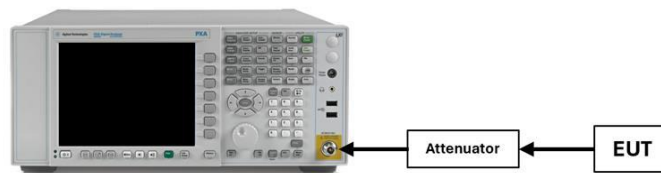
Figure 7-1. Test Instrument & Measurement Setup
