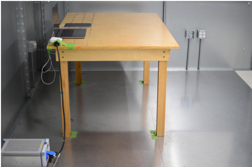
Figure 4: AC Line Conducted Emissions (Side View)
