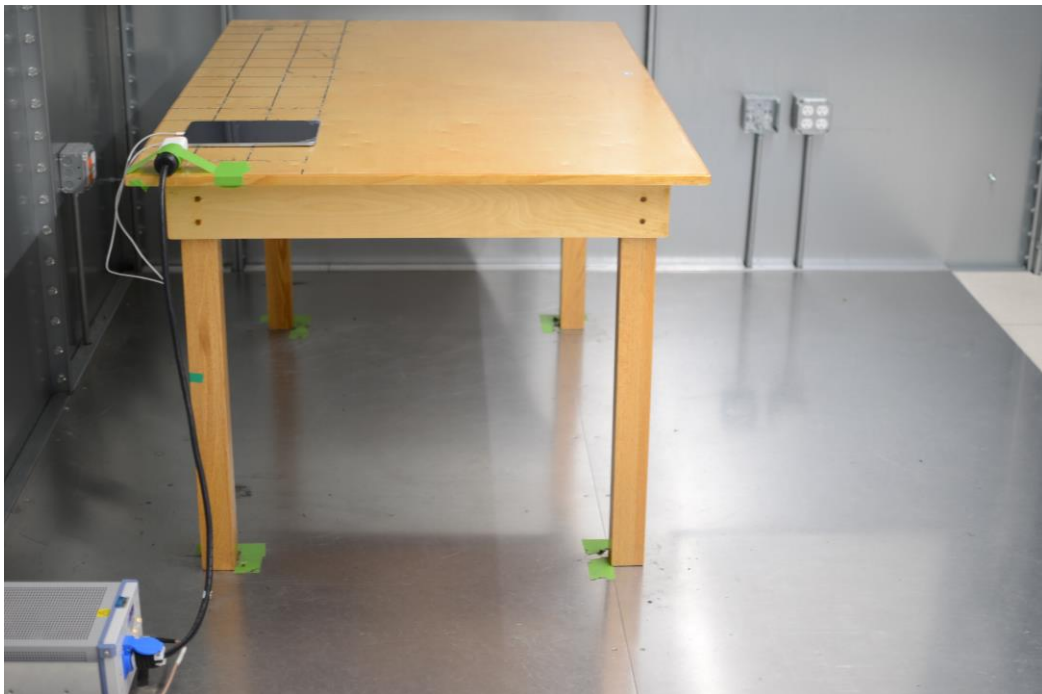
Figure 2: AC Line Conducted Emissions (Side View)
