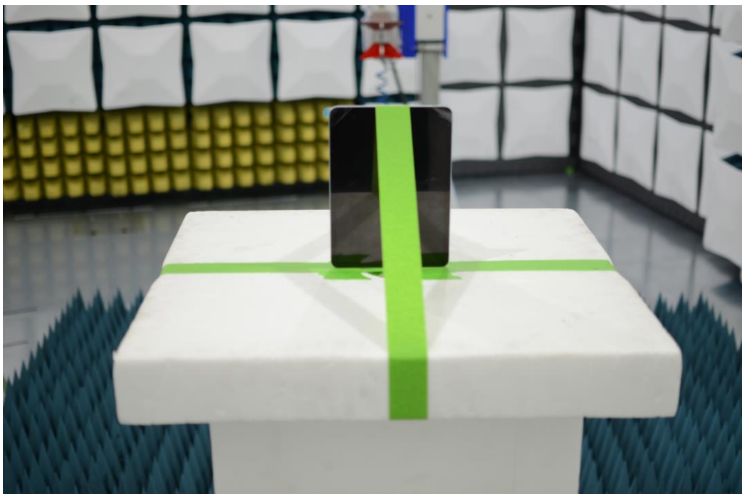
Figure 10: 1-18GHz Test Setup (Rear View)
