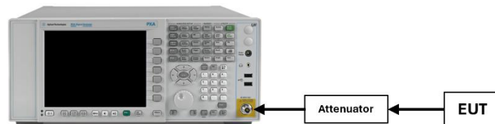
Figure 7-5. Test Instrument & Measurement Setup
