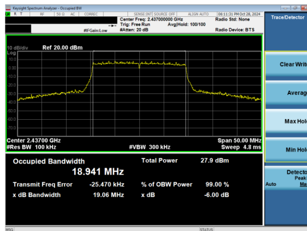
Plot 7-4. 6dB BW & 99% OBW Plot Antenna 1a (802.11ax OFDMA – RU242 – Ch. 6)
