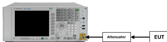
Figure 7-5. Test Instrument & Measurement Setup
