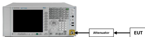
Figure 7-4. Test Instrument & Measurement Setup
