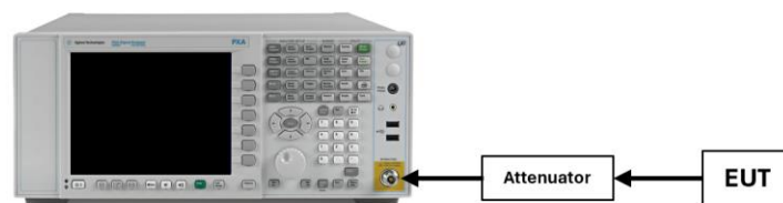
Figure 7-5. Test Instrument & Measurement Setup
