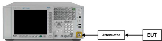
Figure 7-1. Test Instrument & Measurement Setup
