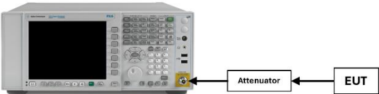
Figure 7-4. Test Instrument & Measurement Setup
