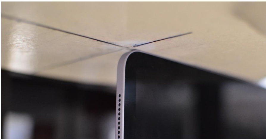
SAR Test Setup Photo 8: Body, Left Edge at 0.0 cm – Antenna 1a/1b/2a/2b
