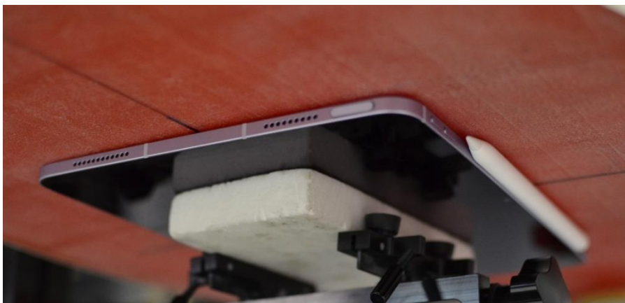
Wireless Power Transfer (wPT) Test Setup Photo 9: Body, Back Side at 0.0 cm
