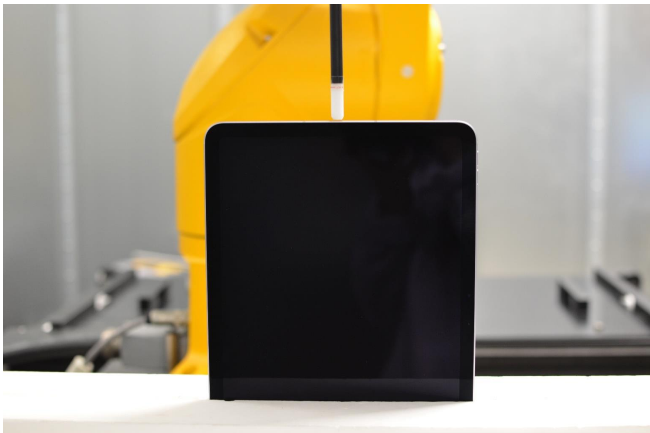
Near Field Power Density Test Setup 17: Top Edge at 2mm – Antenna 1b/3a/3c
