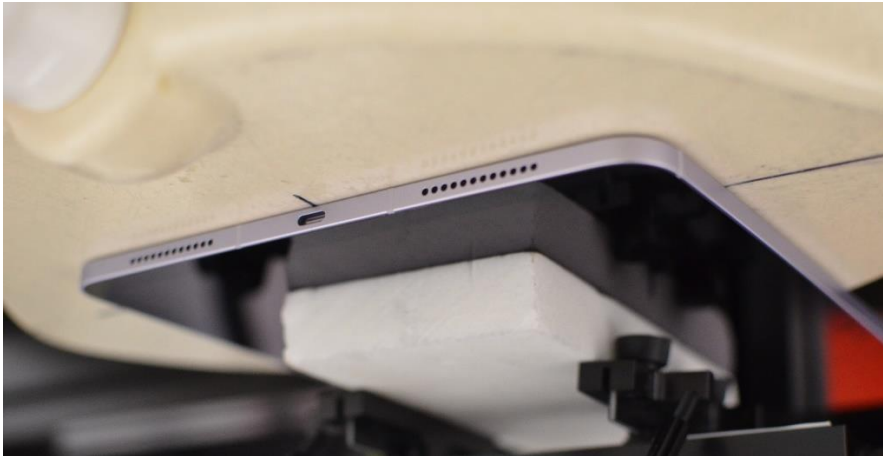
SAR Test Setup Photo 2: Body, Back Side at 0.0 cm – Antenna 1a/1b/2a/2b
