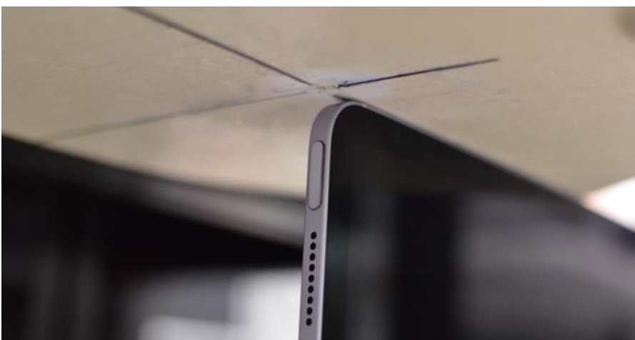
SAR Test Setup Photo 5: Body, Right Edge at 0.0 cm – Antenna 3a/3b/3c/4
