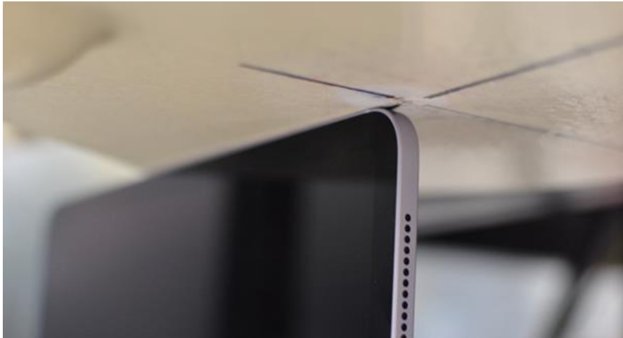
SAR Test Setup Photo 7: Body, Left Edge at 0.0 cm – Antenna 3a/3b/3c/4
