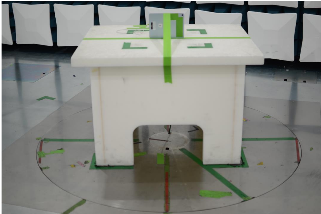
Figure 9: 30MHz-1GHz Test Setup (Front View)
