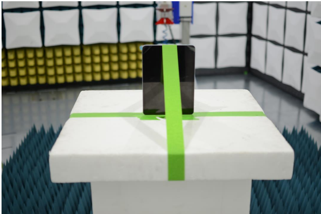
Figure 6: 1-18GHz Test Setup (Rear View)
