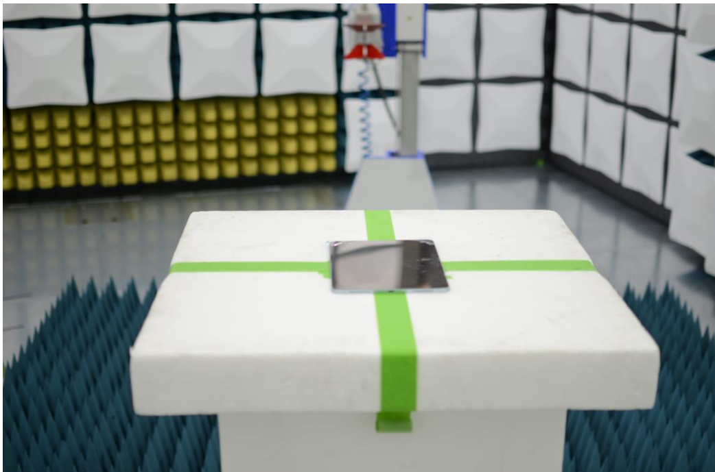
Figure 2: 1-18GHz Test Setup (Rear View)
