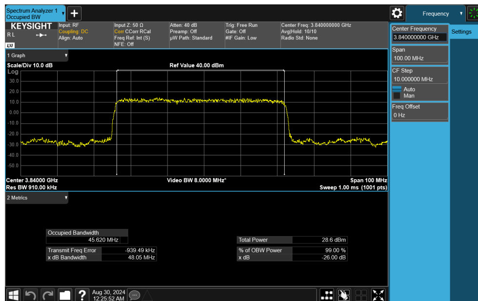
Plot 7-81. Occupied Bandwidth Plot (NR Band n77 C-Band - 50MHz DFT-s-OFDM \pi/2 BPSK - Full RB)
