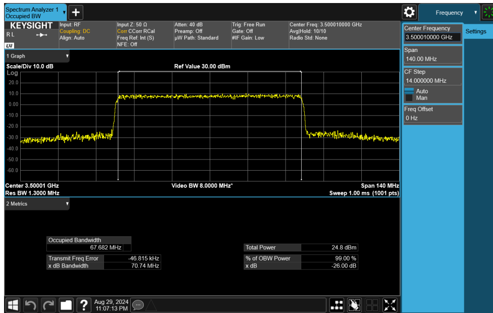
Plot 7-39. Occupied Bandwidth Plot (NR Band n77 DoD-Band - 70MHz CP-OFDM 64-QAM - Full RB)
