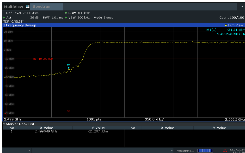
Plot 7-256. Lower Band Edge Plot (LTE Band 7 - 5MHz QPSK – Full RB)
