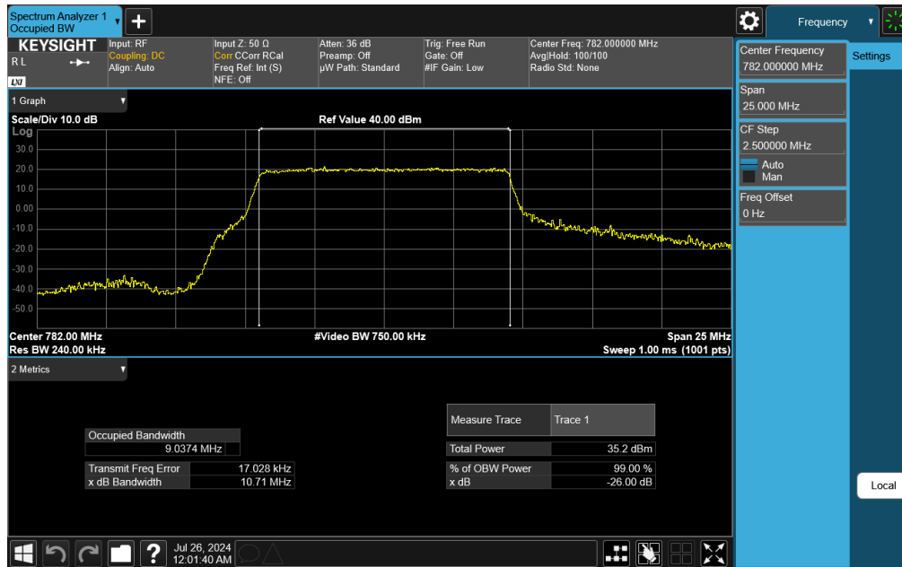
Plot 7-61. Occupied Bandwidth Plot (LTE Band 13 - 10MHz QPSK - Full RB)
