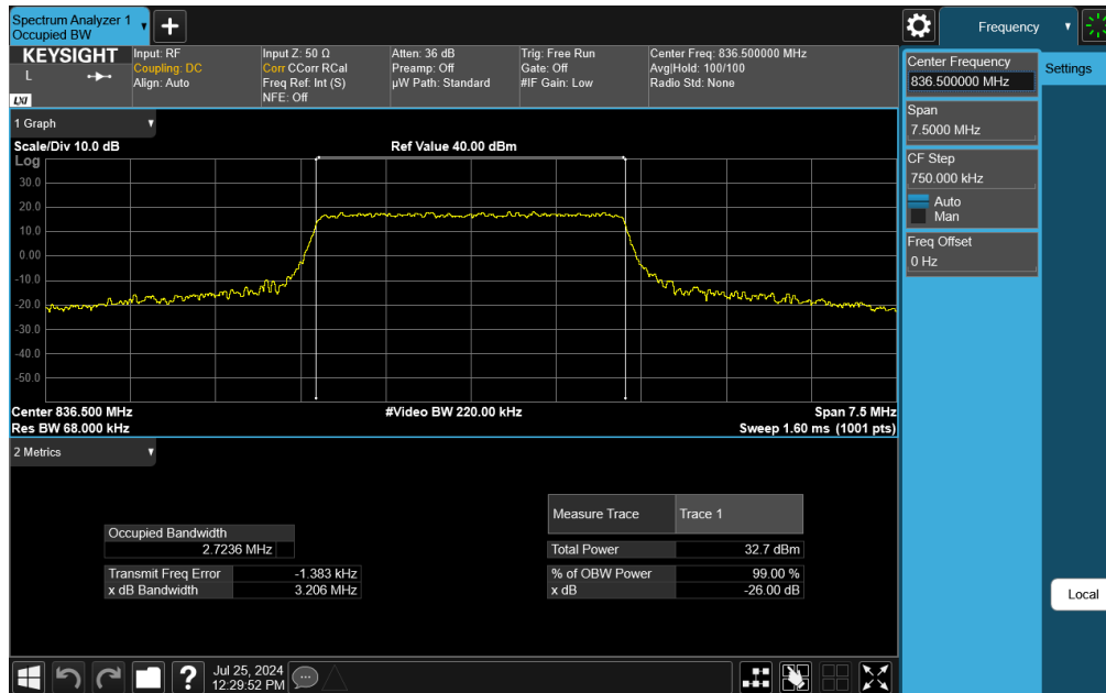
Plot 7-7. Occupied Bandwidth Plot (LTE Band 26/5 - 3MHz 64-QAM - Full RB Configuration)
