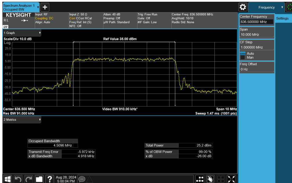
Plot 7-21. Occupied Bandwidth Plot (NR Band n26/n5 - 5MHz n5 DFT-s-OFDM \pi/2 BPSK - Full RB Configuration)
