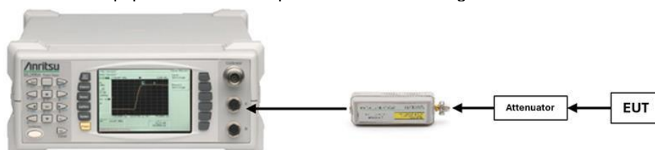
Figure 7-2. Test Instrument & Measurement Setup
