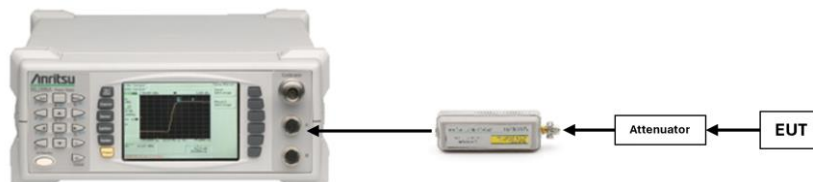
Figure 7-2. Test Instrument & Measurement Setup
