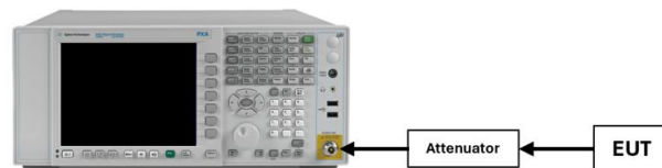
Figure 7-3. Test Instrument & Measurement Setup
