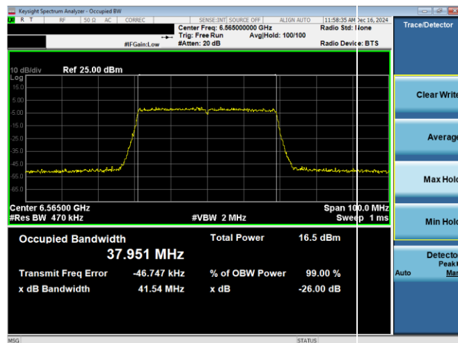
Plot 7-46. 26dB & 99% Bandwidth Plot Antenna WF8 (40MHz 802.11ax RU484 (UNII Band 7) – Ch. 123)
