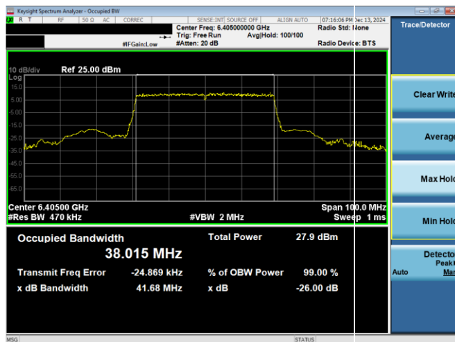
Plot 7-62. 26dB & 99% Bandwidth Plot Antenna WF7a (40MHz 802.11ax RU484 (UNII Band 5) – Ch. 91)
