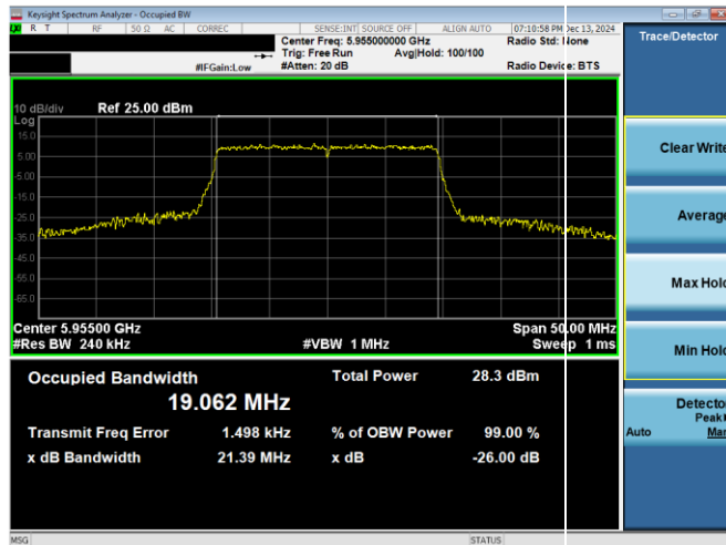
Plot 7-61. 26dB & 99% Bandwidth Plot Antenna WF7a (20MHz 802.11ax RU242 (UNII Band 5) – Ch. 1)
