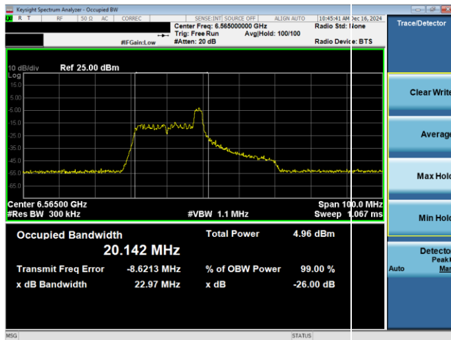
Plot 7-42. 26dB & 99% Bandwidth Plot Antenna WF8 (40MHz 802.11ax RU26 (UNII Band 7) – Ch. 123)
