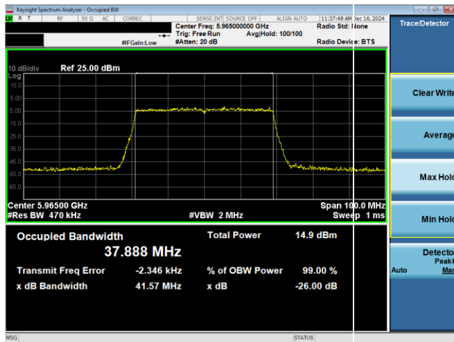
Plot 7-30. 26dB & 99% Bandwidth Plot Antenna WF8 (40MHz 802.11ax RU484 (UNII Band 5) – Ch. 3)
