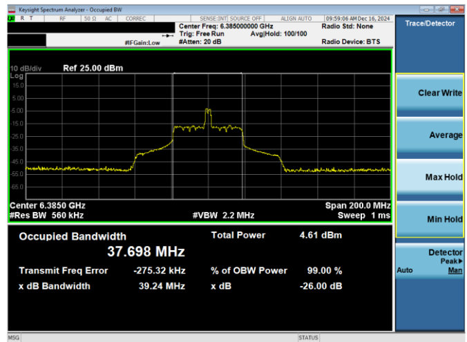
Plot 7-27. 26dB & 99% Bandwidth Plot Antenna WF8 (80MHz 802.11ax RU26 (UNII Band 5) – Ch. 87)
