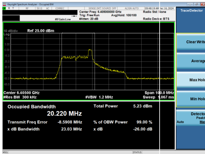
Plot 7-26. 26dB & 99% Bandwidth Plot Antenna WF8 (40MHz 802.11ax RU26 (UNII Band 5) – Ch. 91)
