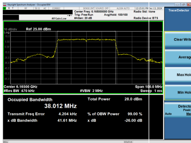
Plot 7-6. 26dB & 99% Bandwidth Plot Antenna WF8 (40MHz 802.11ax RU484 (UNII Band 5) – Ch. 43)
