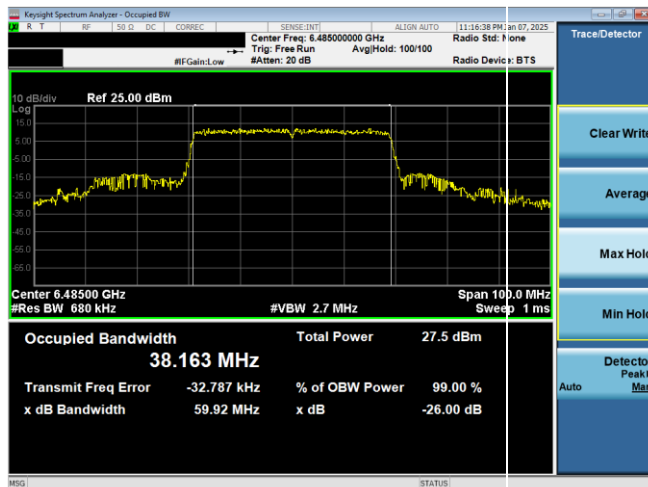
Plot 7-14. 26dB & 99% Bandwidth Plot Antenna WF8 (40MHz 802.11ax RU484 (UNII Band 6) – Ch. 107)
