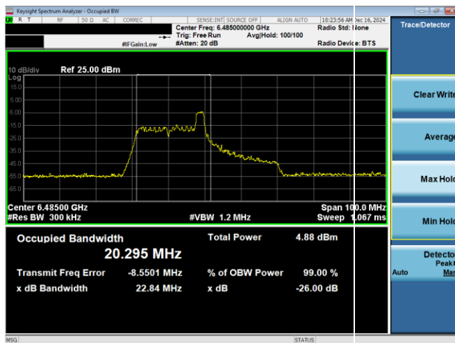
Plot 7-34. 26dB & 99% Bandwidth Plot Antenna WF8 (40MHz 802.11ax RU26 (UNII Band 6) – Ch. 107)
