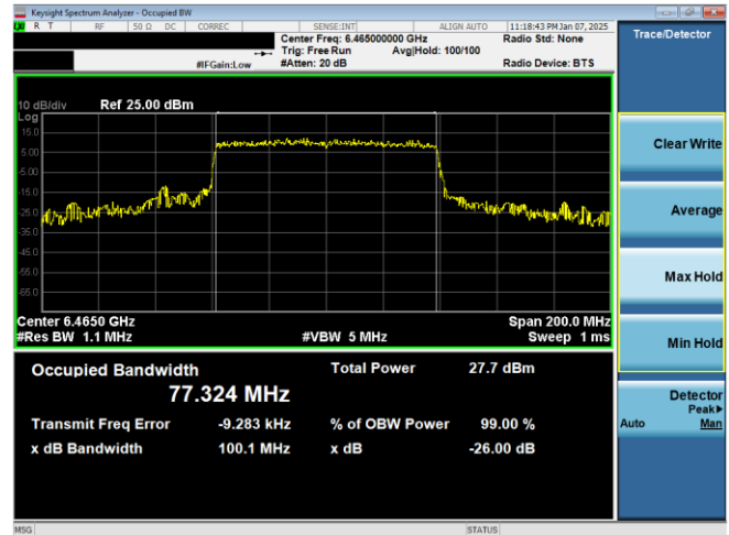
Plot 7-15. 26dB & 99% Bandwidth Plot Antenna WF8 (80MHz 802.11ax RU996 (UNII Band 6) – Ch. 103)
