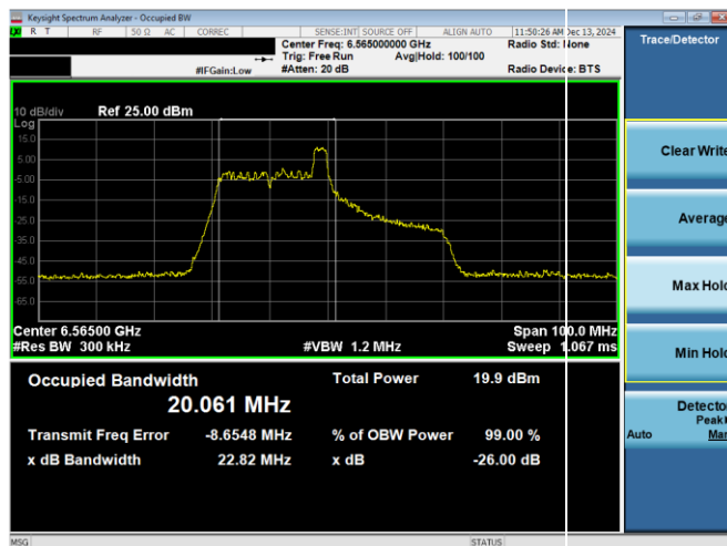
Plot 7-18. 26dB & 99% Bandwidth Plot Antenna WF8 (40MHz 802.11ax RU26 (UNII Band 7) – Ch. 123)
