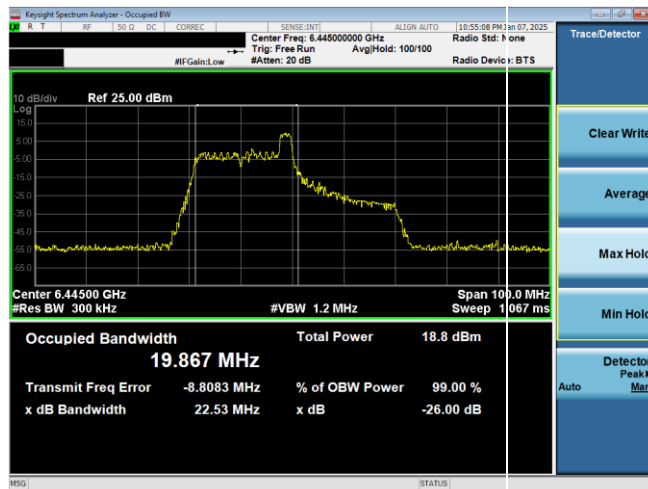
Plot 7-10. 26dB & 99% Bandwidth Plot Antenna WF8 (40MHz 802.11ax RU26 (UNII Band 6) – Ch. 99)
