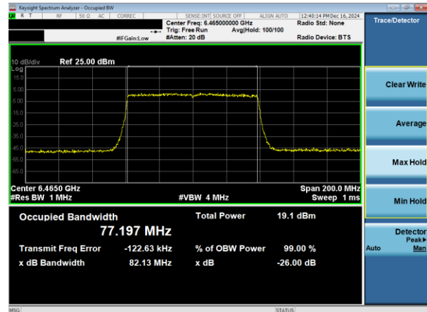
Plot 7-19. 26dB & 99% Bandwidth Plot Antenna WF8 (80MHz 802.11ax (UNII Band 6) – Ch. 103)
