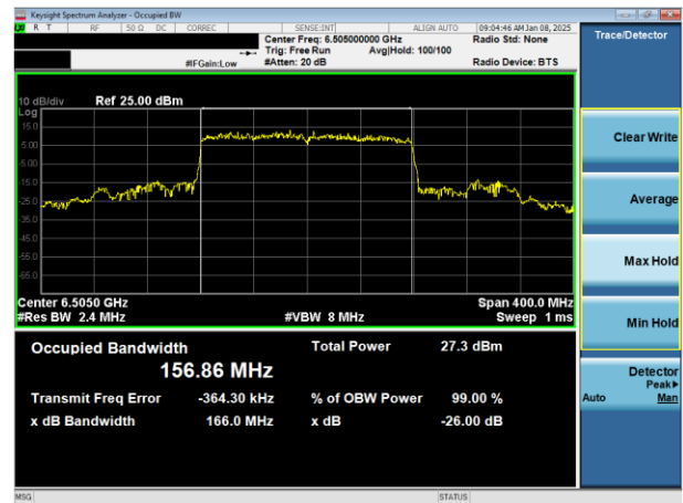
Plot 7-36. 26dB & 99% Bandwidth Plot Antenna WF7a (160MHz 802.11ax (UNII Band 6) – Ch. 111)
