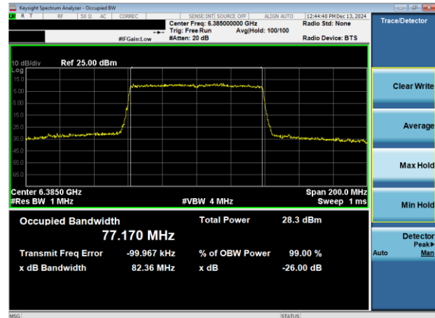
Plot 7-3. 26dB & 99% Bandwidth Plot Antenna WF8 (80MHz 802.11ax (UNII Band 5) – Ch. 87)
