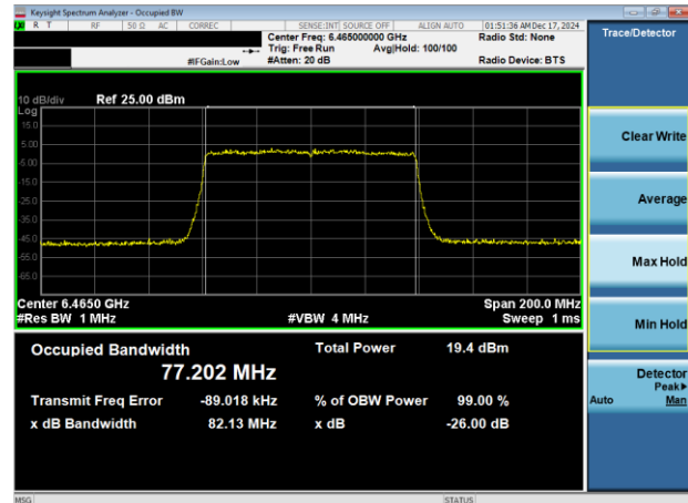
Plot 7-47. 26dB & 99% Bandwidth Plot Antenna WF7a (80MHz 802.11ax (UNII Band 6) – Ch. 103)
