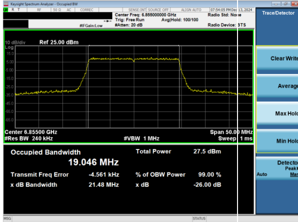
Plot 7-37. 26dB & 99% Bandwidth Plot Antenna WF7a (20MHz 802.11ax (UNII Band 7) – Ch. 181)
