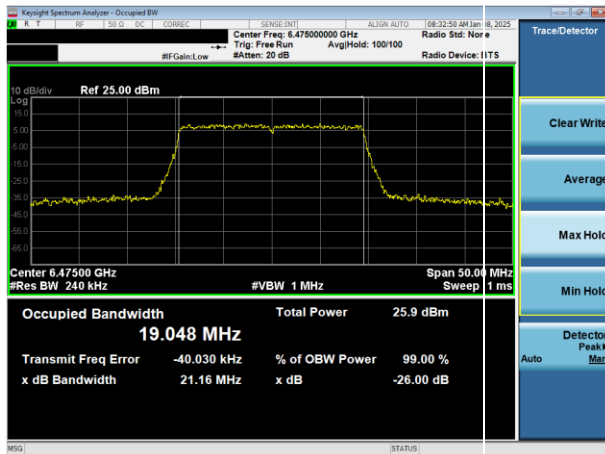
Plot 7-33. 26dB & 99% Bandwidth Plot Antenna WF7a (20MHz 802.11ax (UNII Band 6) – Ch. 105)
