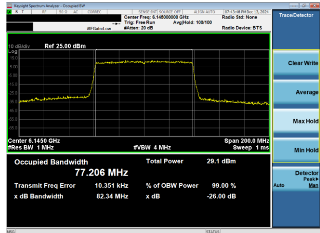
Plot 7-31. 26dB & 99% Bandwidth Plot Antenna WF7a (80MHz 802.11ax (UNII Band 5) – Ch. 39)
