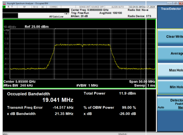
Plot 7-41. 26dB & 99% Bandwidth Plot Antenna WF7a (20MHz 802.11ax (UNII Band 5) – Ch. 1)
