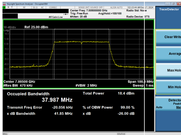
Plot 7-54. 26dB & 99% Bandwidth Plot Antenna WF7a (40MHz 802.11ax (UNII Band 8) – Ch. 211)
