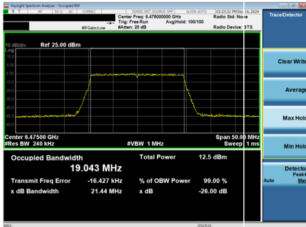
Plot 7-17. 26dB & 99% Bandwidth Plot Antenna WF8 (20MHz 802.11ax (UNII Band 6) – Ch. 105)
