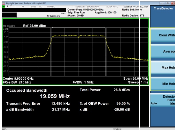
Plot 7-1. 26dB & 99% Bandwidth Plot Antenna WF8 (20MHz 802.11ax (UNII Band 5) – Ch. 1)
