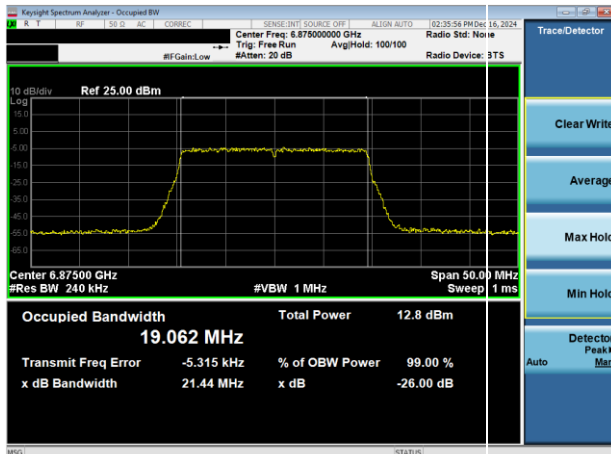
Plot 7-21. 26dB & 99% Bandwidth Plot Antenna WF8 (20MHz 802.11ax (UNII Band 7) – Ch. 185)
