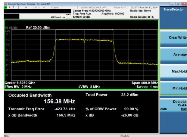
Plot 7-52. 26dB & 99% Bandwidth Plot Antenna WF7a (160MHz 802.11ax (UNII Band 7) – Ch. 175)
