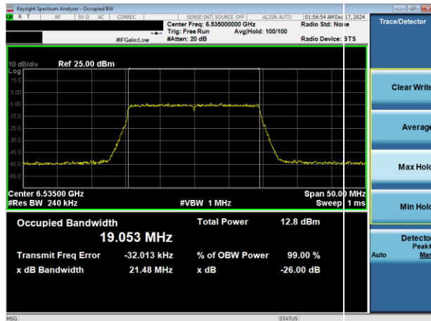
Plot 7-49. 26dB & 99% Bandwidth Plot Antenna WF7a (20MHz 802.11ax (UNII Band 7) – Ch. 117)
