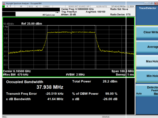
Plot 7-30. 26dB & 99% Bandwidth Plot Antenna WF7a (40MHz 802.11ax (UNII Band 5) – Ch. 43.)
