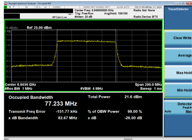
Plot 7-55. 26dB & 99% Bandwidth Plot Antenna WF7a (80MHz 802.11ax (UNII Band 8) – Ch. 199)
