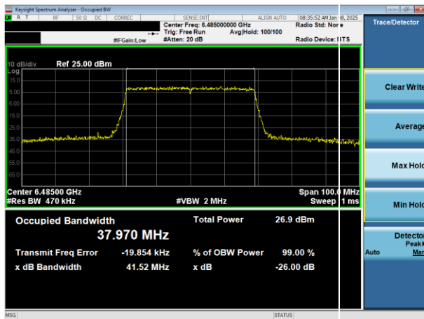
Plot 7-34. 26dB & 99% Bandwidth Plot Antenna WF7a (40MHz 802.11ax (UNII Band 6) – Ch. 107)
