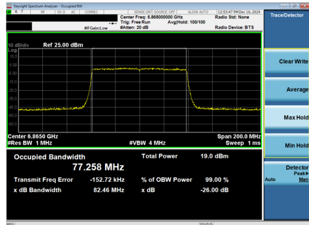
Plot 7-23. 26dB & 99% Bandwidth Plot Antenna WF8 (80MHz 802.11ax (UNII Band 7) – Ch. 183)
