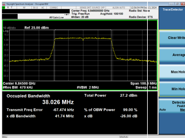
Plot 7-10. 26dB & 99% Bandwidth Plot Antenna WF8 (40MHz 802.11ax (UNII Band 7) – Ch. 179)
