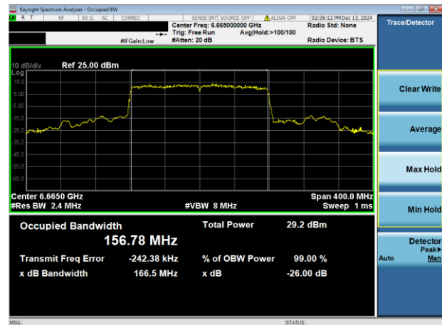
Plot 7-12. 26dB & 99% Bandwidth Plot Antenna WF8 (160MHz 802.11ax (UNII Band 7) – Ch. 143)
