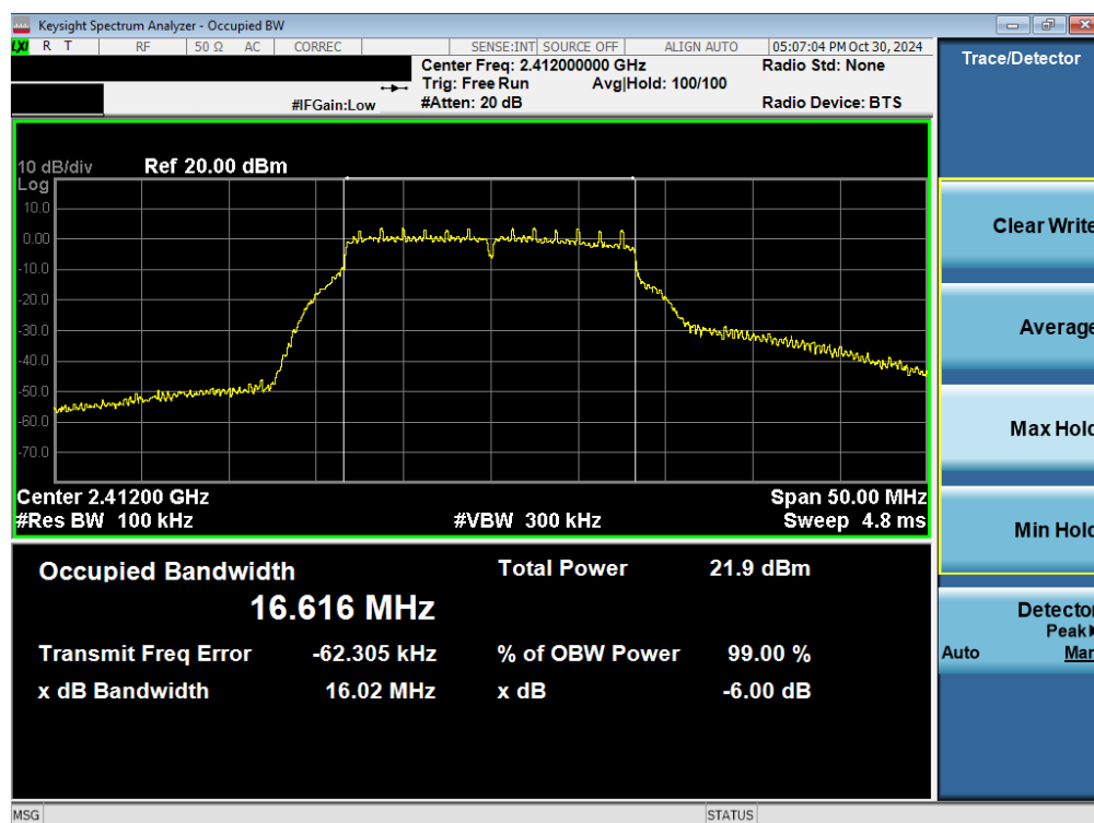
Plot 7-6. 6 dB BW and 99% OBW Plot Antenna WF7b (802.11g – Ch. 1)
