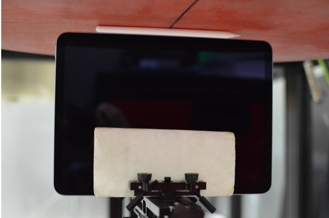
Wireless Power Transfer Test Setup (wPT) Photo 15 – Right Edge at 0 mm
