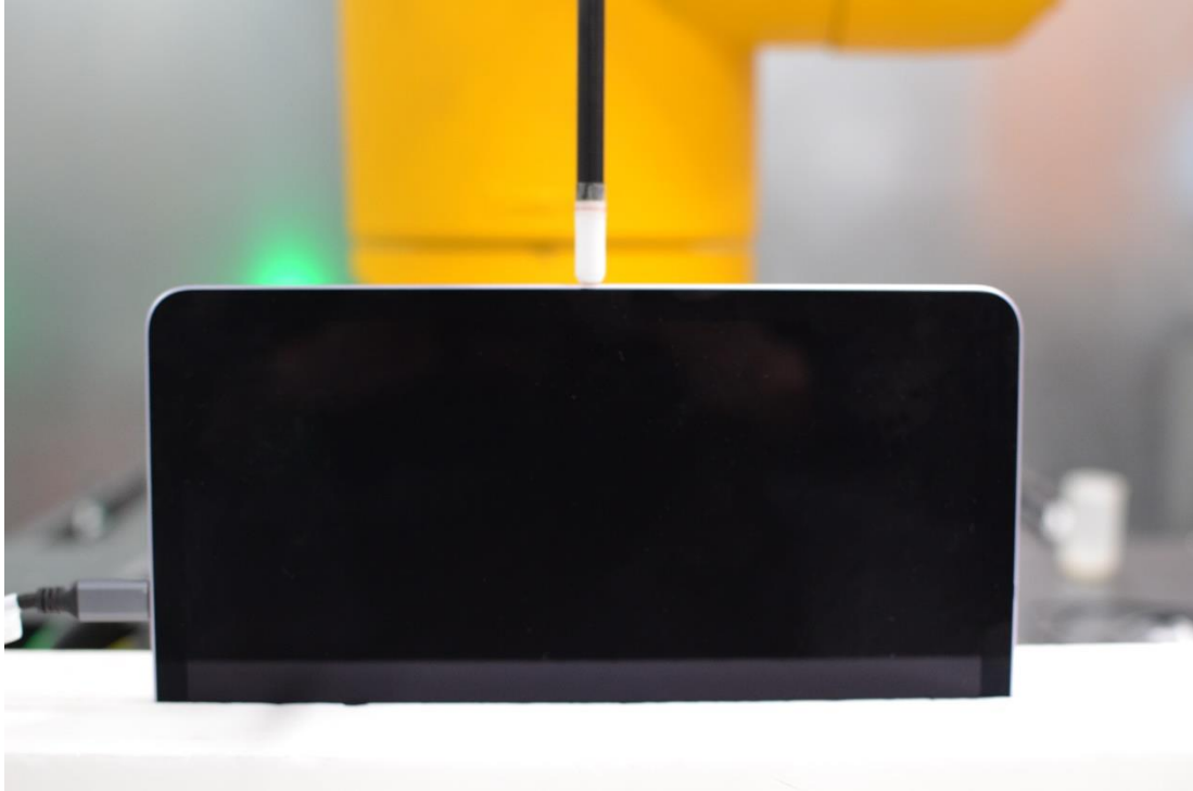
Near Field Power Density Test Setup Photo 11 – Left edge at 2 mm
