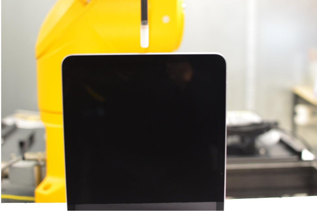
Near Field Power Density Test Setup Photo 7 – Top edge at 9 mm
