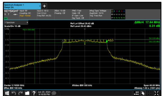
Figure 231 - 802.11n HT20 Maximum 6 dB EBW
