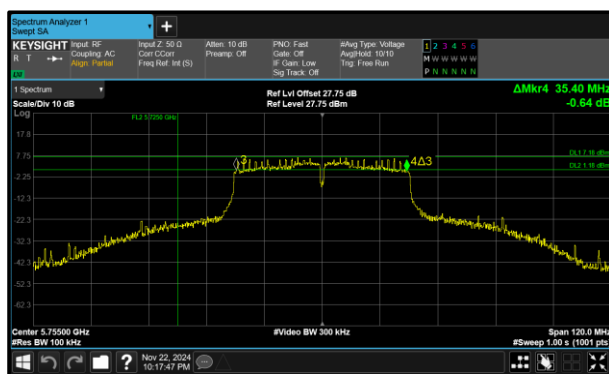
Figure 308 - 802.11n HT40 Minimum 6 dB EBW
