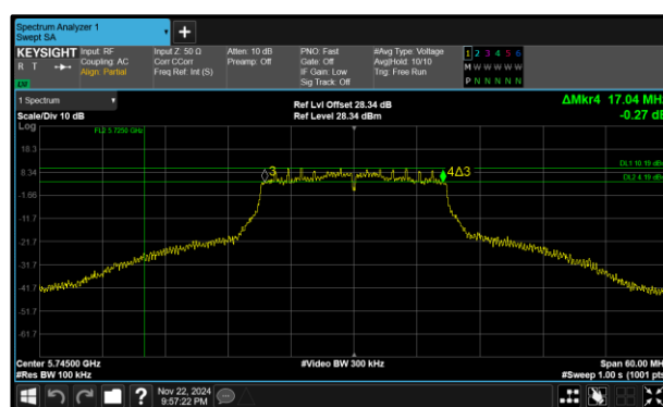
Figure 307 - 802.11n HT20 Maximum 6 dB EBW
