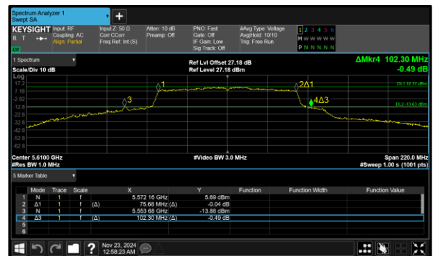
Figure 323 - 802.11ac VHT80 Maximum 26 dB EBW
