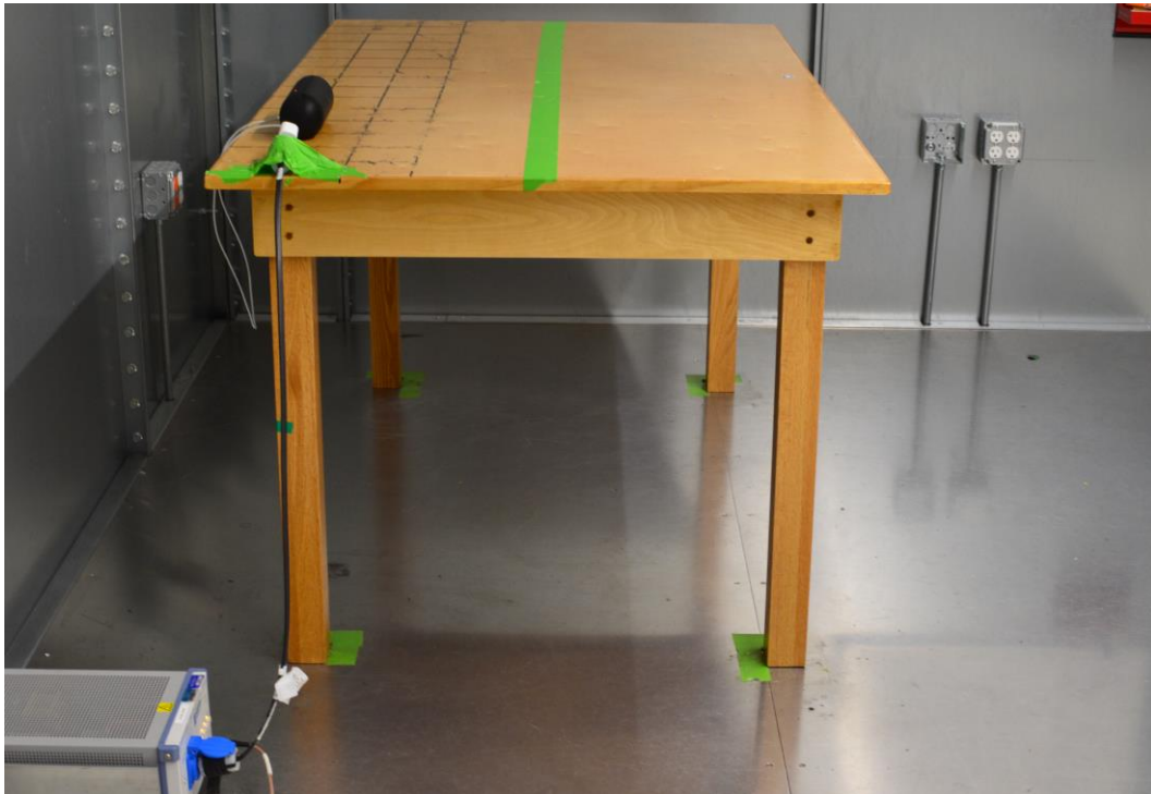
Figure 2: AC Line Conducted Emissions (Side View)
