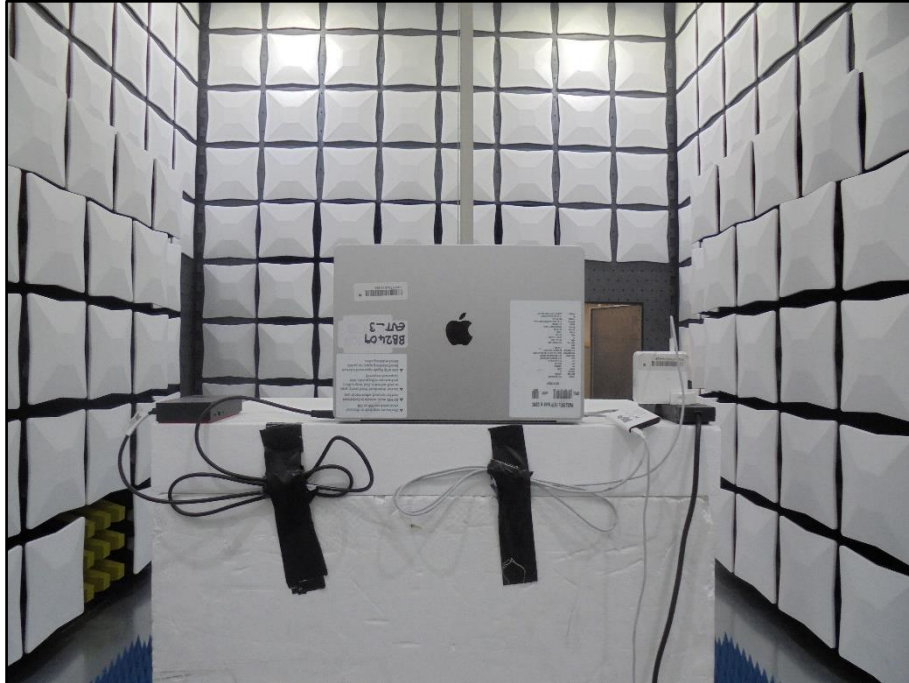
Figure 3 - Radiated Disturbance - Above 1 GHz
