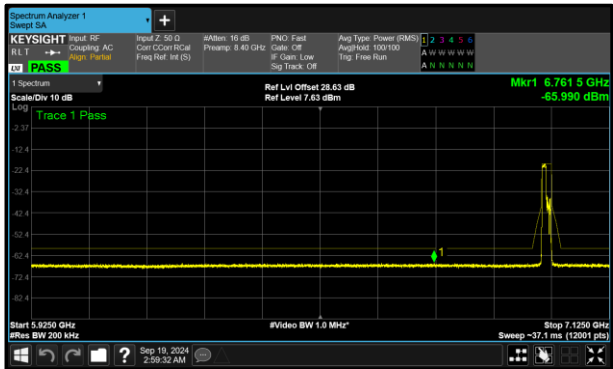
Figure 378 - B (Core 1) 802.11ax HE20 RU106 LPI 6995 MHz (CH209)
