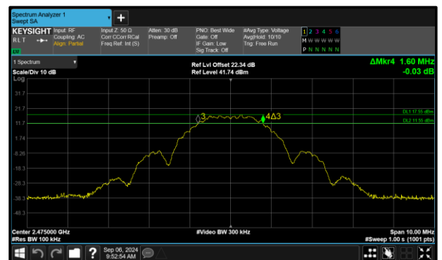
Figure 22 - Core 0 (A) 2475 MHz (CH25) 6 dB Bandwidth
