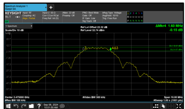
Figure 28 - Core 1 (B) 2475 MHz (CH25) 6 dB Bandwidth
