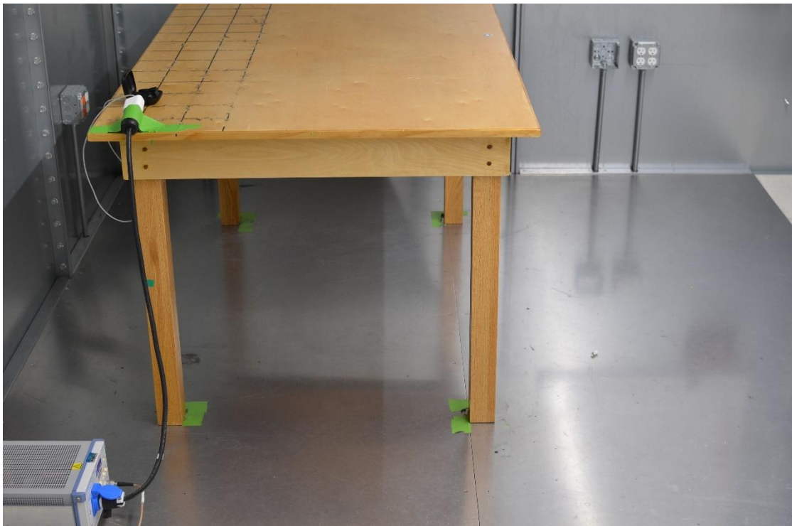
Figure 2: AC Line Conducted Emissions (Side View)
