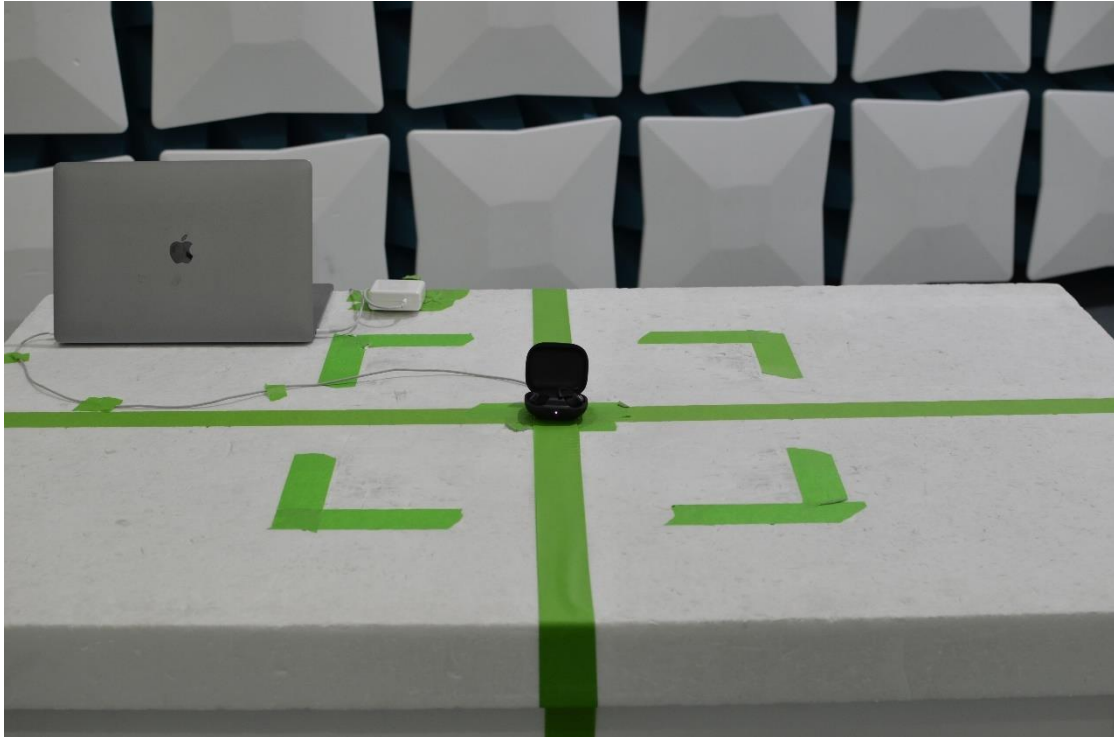
Figure 17: 30MHz-1GHz Test Setup (Front View)
