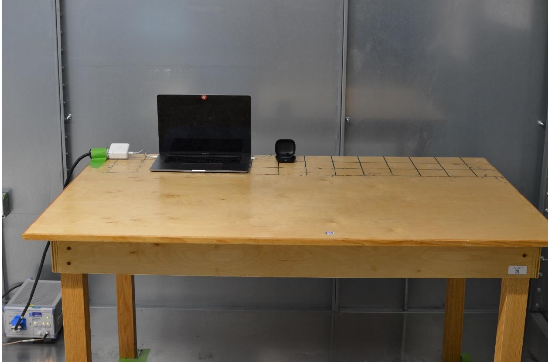
Figure 3: AC Line Conducted Emissions (Front View)
