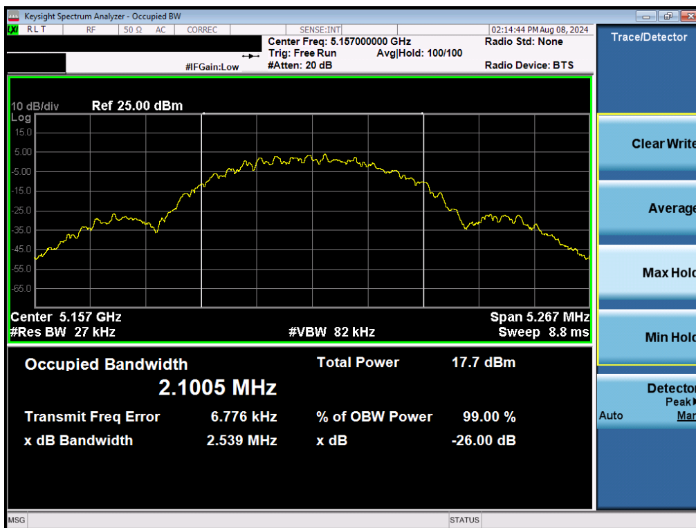
Plot 7-4. 26dB BW & 99% OBW (NB UNII LE2M – 5157MHz)
