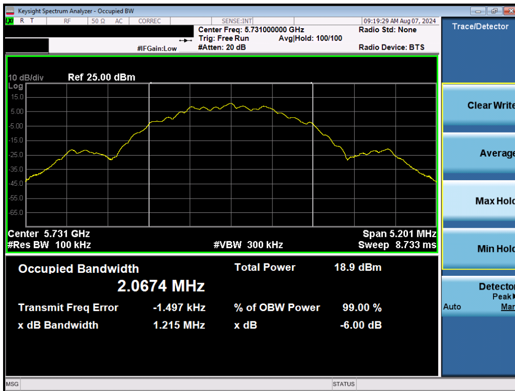
Plot 7-22. 6dB BW & 99% OBW (NB UNII LE2M – 5731MHz)
