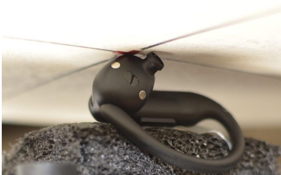
SAR Test Setup Photo 1: Head position, Right Earbud, 0 mm
