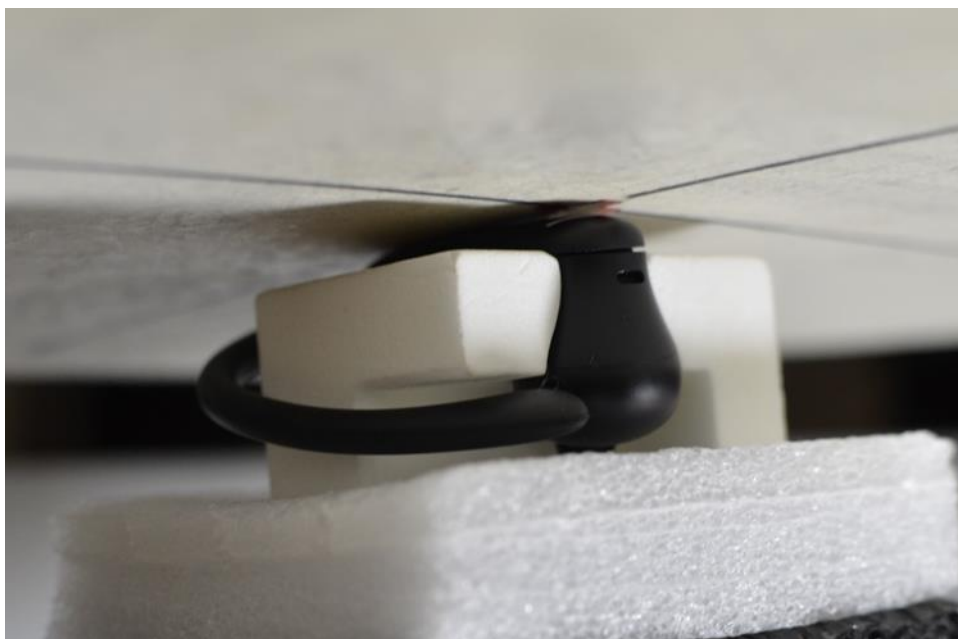
SAR Test Setup Photo 2: Body-Worn, Logo position, Right Earbud, 0 mm
