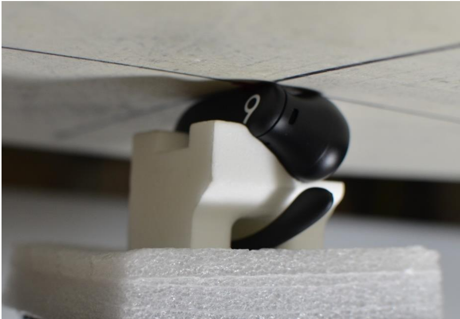
SAR Test Setup Photo 4: Body-Worn, Non-button position, Right Earbud, 0 mm
