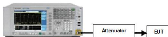
Figure 7-3. Test Instrument & Measurement Setup
