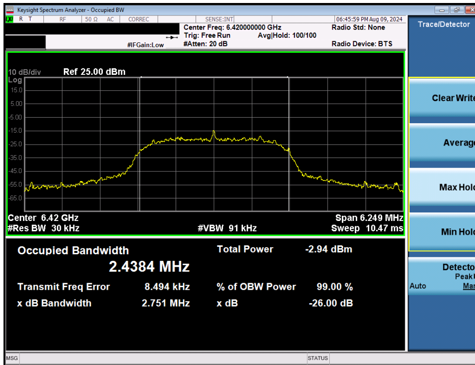
Plot 7-15. 26dB BW & 99% OBW (NB UNII HDRp4 – 6420MHz)
