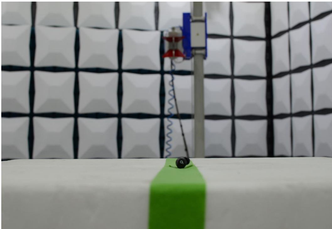
Figure 12: 1-18GHz Test Setup (Rear View)
